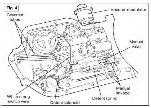
4. There are (3) 1/4-20 and (8) 5/16-18 bolts holding the valve body. Remove all but one valve body bolt and disconnect the spark control switch wire if present. Hold the valve body in place and remove the last bolt. Lower the valve body while at the same time pulling straight down on the governor tubes (See Fig. 5). Place the valve body in the oil pan to avoid contamination.
