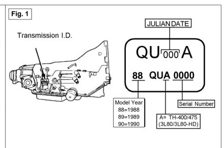
If the I.D. tag is unreadable or missing you will have to remove the oil pan and valve body from the transmission to determine if your transmission has an early or late style case (See Fig. 2). The manufacturing date check applies only to 1988 transmissions, this kit will work correctly in all subsequent application years specified in the heading of these instructions.
