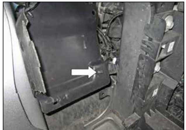
p. Disengage the final plastic clip at the bottom of the OEM inlet duct and remove the duct.
