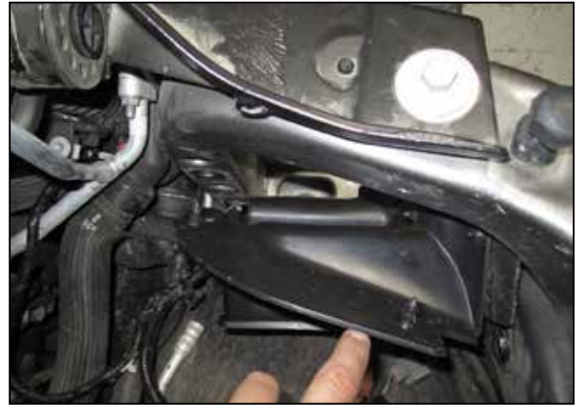
n. Disengage the two plastic clips at the top of the OEM air box inlet duct.
