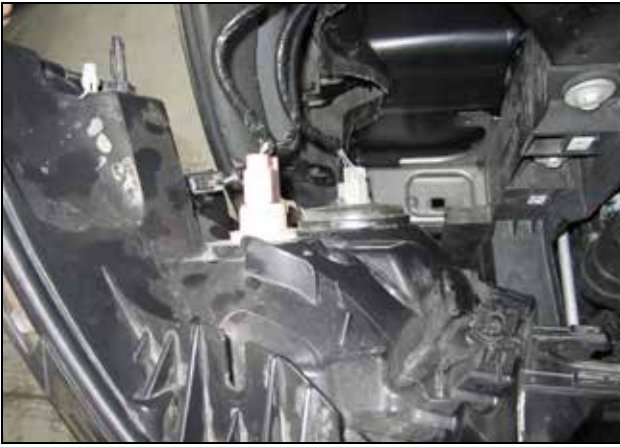
k. Firmly pull out on the headlight and disconnect all 3 plugs.
