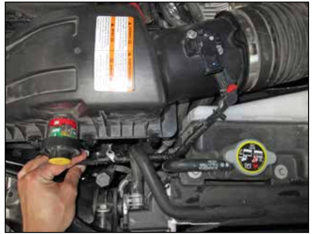
b. Unplug the MAF sensor and unclip the wire harness from the air box.
