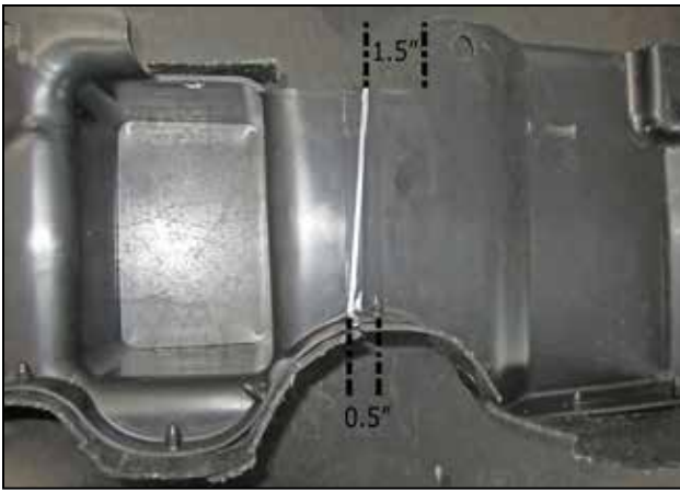
q. Measure and mark the OEM inlet duct as shown.
