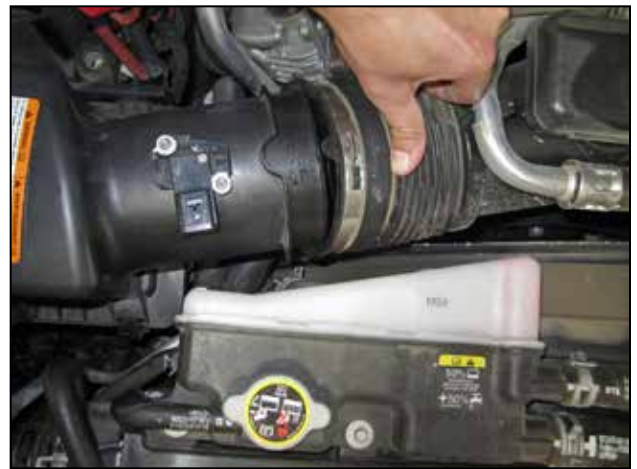
d. Disconnect the intake hose from the air box neck.
