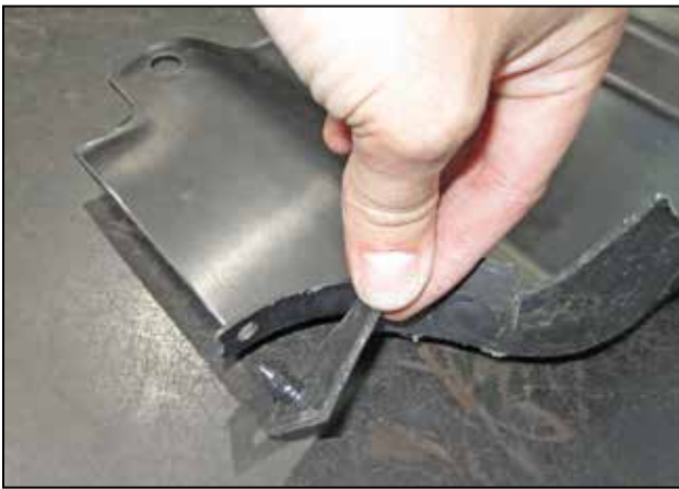
s. After cutting the duct, remove the plastic clip as shown.
