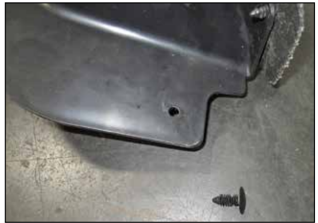
t. Remove one of the plastic clips from the top half of the OEM inlet duct to use during installation.
