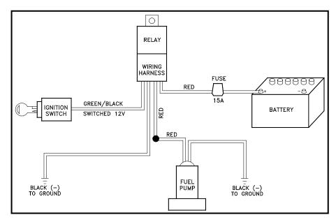
7. Attach the in-line fuse holder to the remaining Red wire. After attaching the fuse holder, insert 15A fuse and connect to the positive side of battery.
