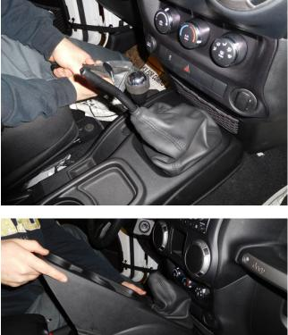
3) Unscrew the square secure plate holding the rubber boot over the shifter. Then remove the rubber boot.
