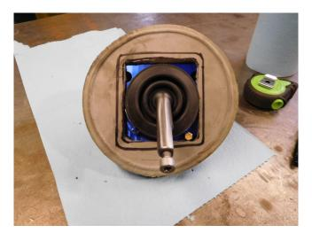
12) Use a ratchet with a T30 torx socket to unbolt and remove the stock shifter.
