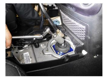
18) Reinstall the rubber boot over the factory shifter stick and secure it to the floor with the factory square flat nut.
