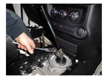
5) Spray some lubricant in the hole where the bolt was removed. Then with a pair of vise grips, clamp onto the stick down low near where the bolt was removed and lightly hit the vise grips with a hammer to pull the shifter stick off of the shifter shaft.
