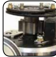
Precision magnetic pickup coil and reluctor.
