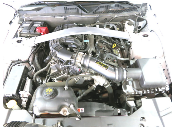
AEM INTAKE INSTALLED
