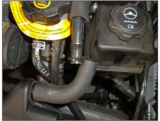
f. Disconnect the rubber breather hose from the plastic breather pipe.
