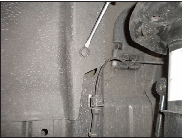
d. Locate and remove the retaining tab at the shock tower with a flat blade screwdriver as shown.
