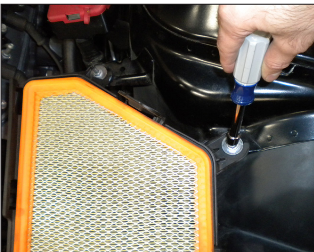
i. To remove the stock lower airbox, remove the 2 retaining nuts near the shock tower bracket (Retain these, they will be used to install the AEM® intake system).
