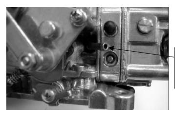
Connect a vacuum hose from this fitting to a vacuum source on the lower manifold.
