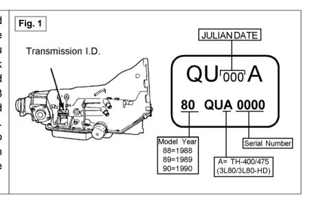
If the I.D. tag is unreadable or missing you will have to remove the oil pan and valve body from the transmission to determine if your transmission has an early or late style case (See Fig. 2). This kit will work correctly in all 1965-1987 TH-400 transmissions.
