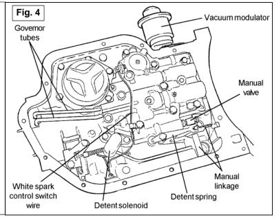
4. There are (3) 1/4-20 and (8) 5/16-18 bolts holding the valve body. Remove all but one valve body bolt and disconnect the spark control switch wire if present. Hold the valve body while at the same time pulling straight down on the governor tubes (See Fig. 5). Place the valve body in the oil pan to avoid contamination.
