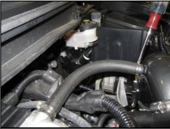
Q. Install the 5/8 hose (N) and two hose clamps (Q) on the PCV vent on the valve cover and the intake tube.
