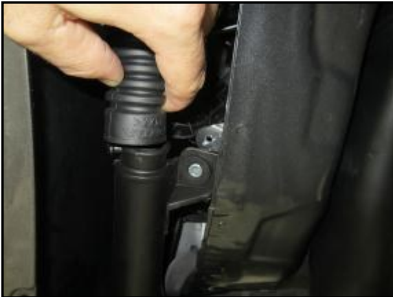
S. Disconnect the sound tube from the resonator.
