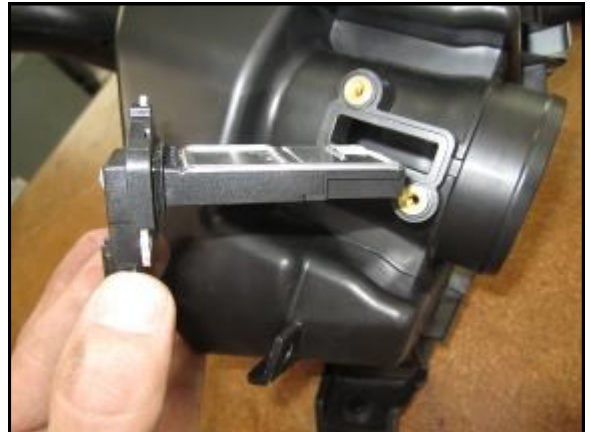
X. Remove the MAF sensor.
