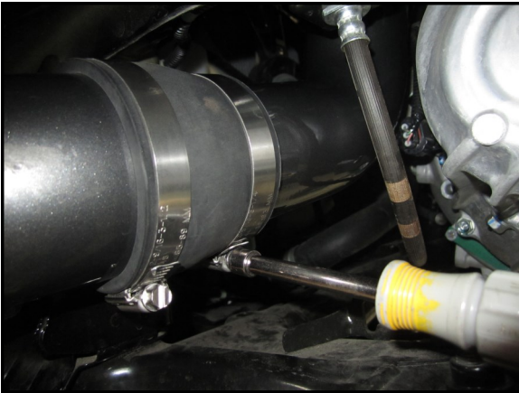
S. Now tighten the two lower clamps.
