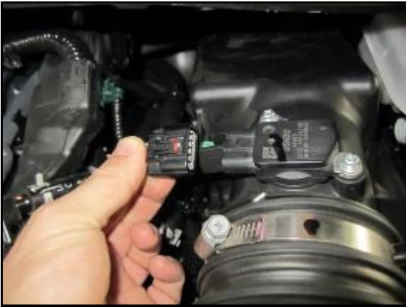
A. Unplug the MAF sensor.
