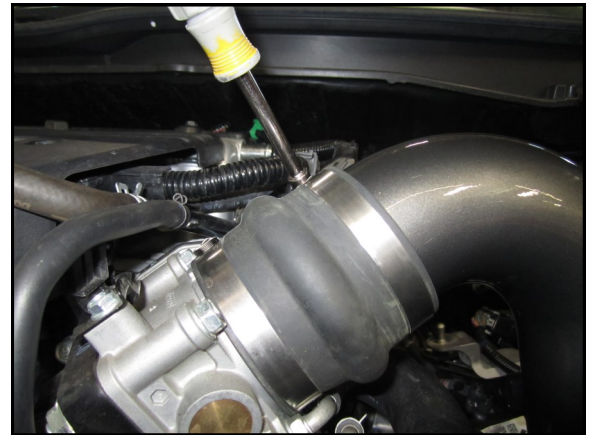
T. Now tighten the upper clamp.
