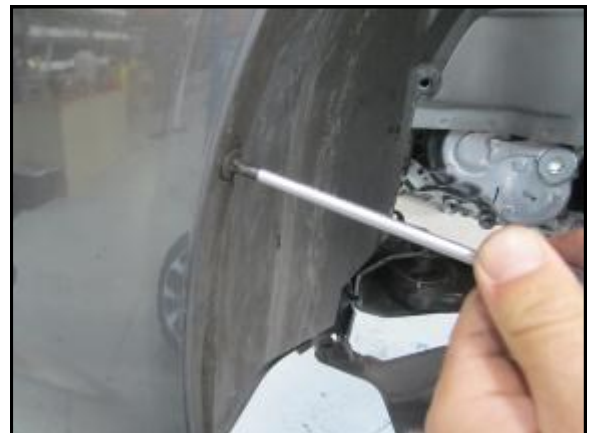
N. Remove the Philips screw.
