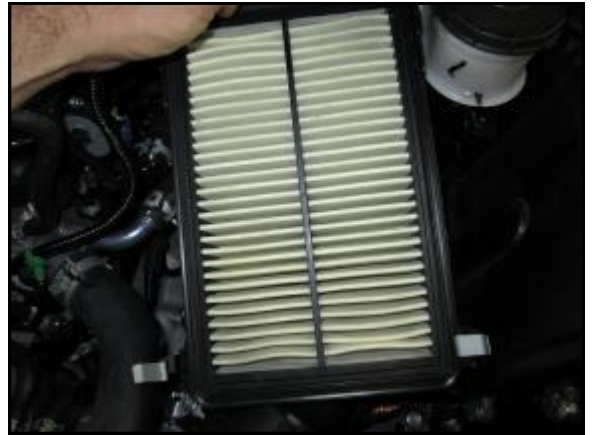
H. Lift up on the back of the lower air box and remove the box.
