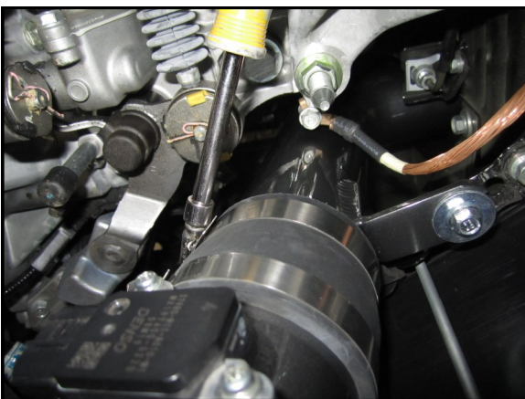
U. Now tighten the final hose clamp.
