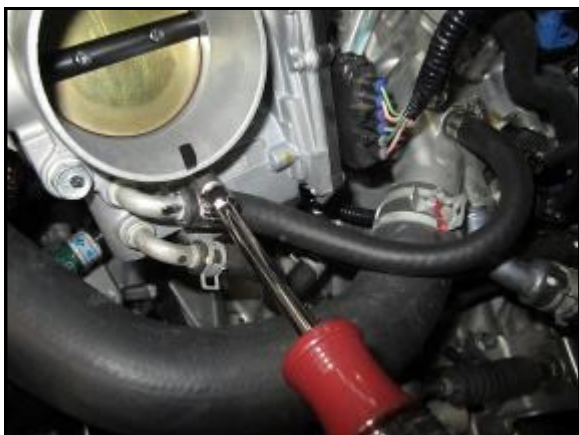
A. Install the provided 10" 5/16 hose (P) and two 1/4" hose clamps (O) on the throttle body and thermostat and tighten the hose clamps as shown.
