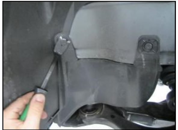
L. Remove the two plastic clips securing the side splash shield.
