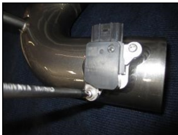
D. Install the MAF sensor in the upper intake tube (A).
