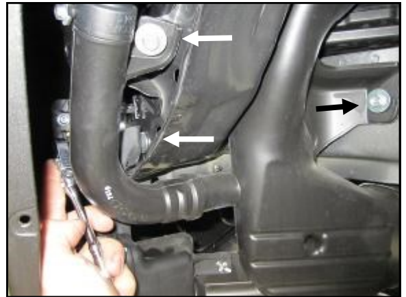
R. Remove the three M6 bolts holding the resonator and sound tube.
