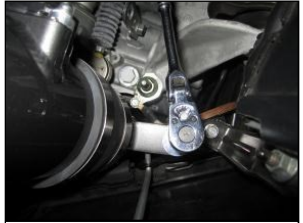
R. Make sure you have proper clearance around the intake system and tighten the M6 bolt on the middle tube bracket.
