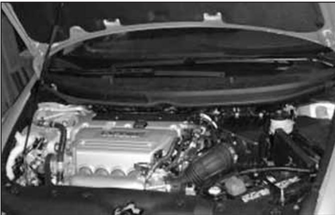
Factory air box system installed
