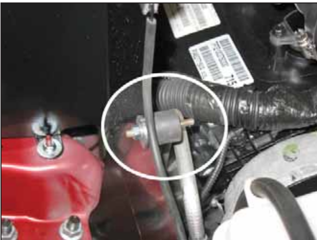
l. Install the rubber mount, fender washer and M6 nut onto the heat shield.
