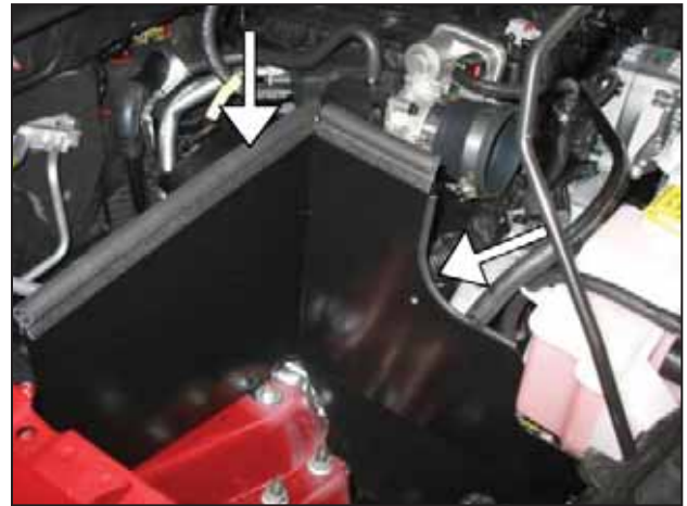
k. Attach the sponge gasket to the top to the heat shield. Attach the rubber edge trim on the radius.
