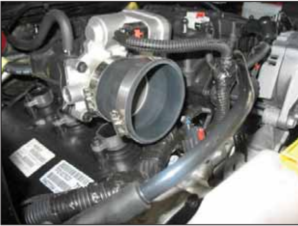
h. Attach the coupler to the throttle body and secure with #44 (9452) and #52 (9452) hose clamp.
