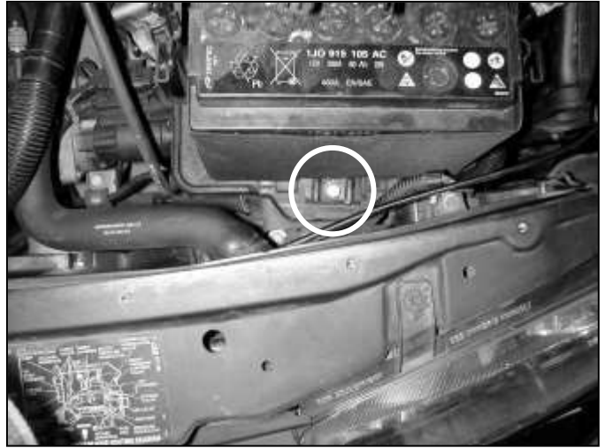
d. Remove the battery hold down bolt and remove the battery from the vehicle.
