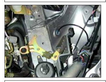
g. Pull up and remove air box from car.
