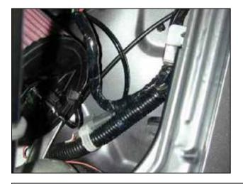
r. Cut and remove the electrical tape on the relay harness to give it more length.
