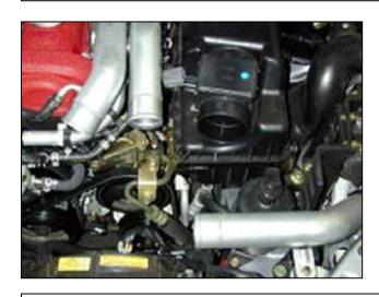
d. Remove the boost pipe elbow and the inlet tube. You will reuse the boost side elbow during the AEM® intake installation.
