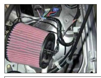
q. Install the air filter and tighten the hose clamp. Insert the IAT sensor into the hole in the end of the air filter. Attach the supplied 6" zip-tie to the IAT and relay harness as shown. Adjust the IAT harness so it does not contact the air filter.
