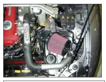
m. Install the supplied AEM® hot pipe using the front and rear stock elbow couplers removed in step 2j. Temporarily install the filter at this time. Check for clearance around the filter and tighten all hose clamps.
