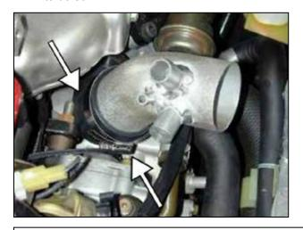
b. Install the supplied 1.75" to 2.25" reducing elbow onto the turbo inlet with the inlet pipe and hose clamps as shown.
