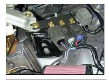
u. Attach the relays to relay bracket using the stock M6 nuts and bolts from the removal in step 2h as shown.
