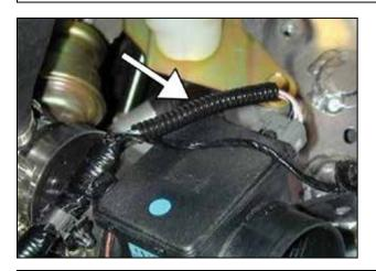
h. Install supplied slit loom to MAF wires as shown.
