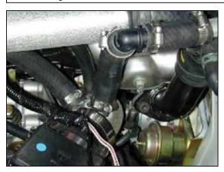
k. Install the supplied 3/4" and 5/16" hoses onto the inlet pipe as shown. Use the supplied spring clamps and screw clamps as shown.
