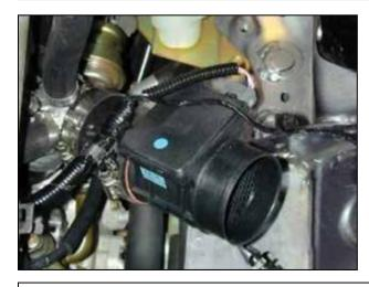
e. Install the MAF assembly from step 3c onto inlet pipe. The MAF bracket will install on to the rubber mount. Secure using the supplied M6 Nylok nut. Reconnect the MAF wiring harness to the MAF adapter assembly.
