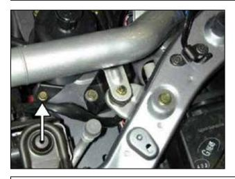
n. Remove the M6 bolt on the power steering reservoir bracket in preparation to install the AEM® heat shield. The M6 bolt will be reused in a later step.
