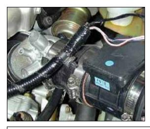
g. Remove the electrical tape as shown.
