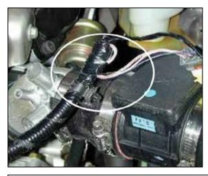
f. Cut the electrical tape holding the MAF sensor wires to the harness to free up additional length. BE CARE-FUL AND ENSURE NO WIRES ARE CUT.
