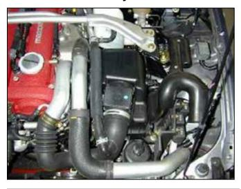
a. Factory air box system installed.
