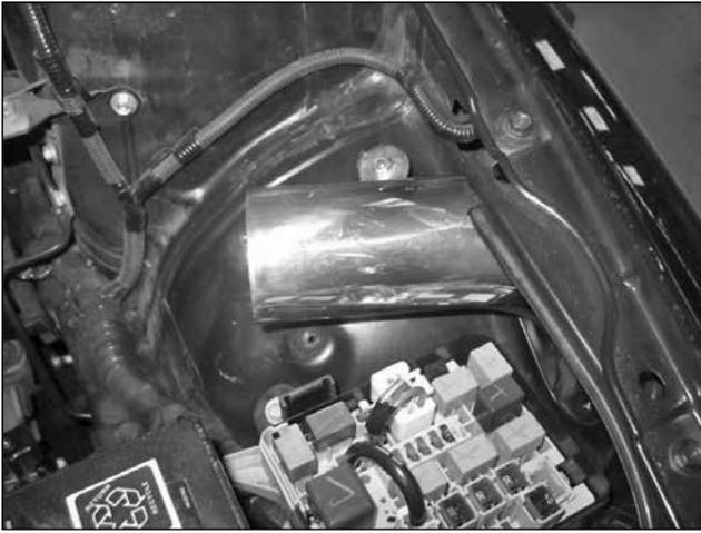
d. Install the lower intake pipe from inside the wheel well (Keep plastic on intake pipe to prevent scratching). Slide upper bracket over rubber mount, loosely secure with 6mm washer and 6mm nut (remove plastic).
