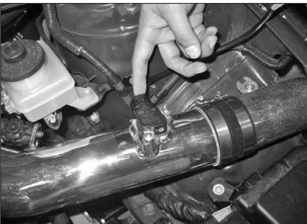
n. Connect the female connector of the ETI module to the MAF sensor installed in the upper intake pipe.
