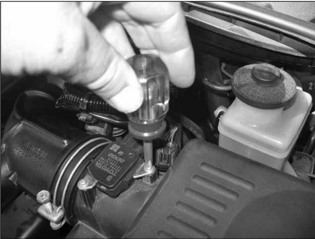
c. Remove the mass airflow sensor from the intake tube (Be sure to keep in a safe place to be used later.).
