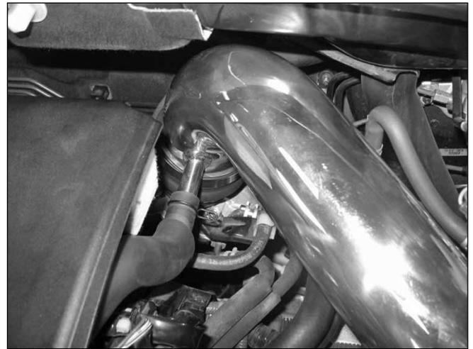
s. Connect the breather hose to the nipple on the upper intake pipe.
