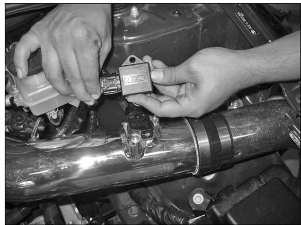
o. Connect the female connector coming from the vehicle to the male connector located on the ETI module.
