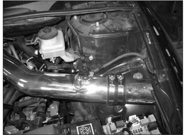
k. Align the upper intake tube with the lower intake tube and slide the coupler over the upper intake tube so that the coupler covers both tubes evenly. Loosely secure the three #48 hose clamps.
