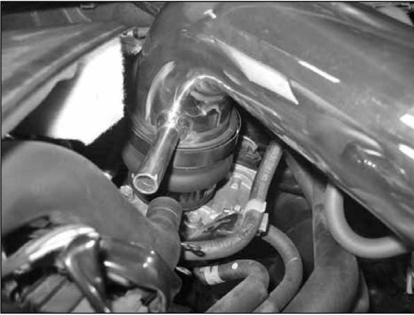
j. Install the upper intake tube into the hump hose connected to the throttle body.
