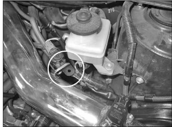
m. Use the screw removed in 2e to secure the VSV and harness bracket (7-7717) to the bracket on the upper intake pipe. Reconnect the short vacuum line.
