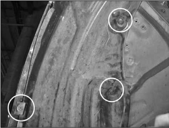
q. Remove the screw and clips holding on the driver side fender liner.
