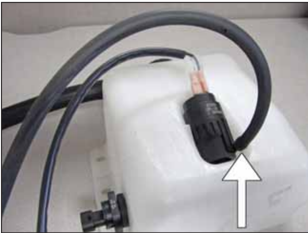
al. Connect the washer fluid hose to the pump.
