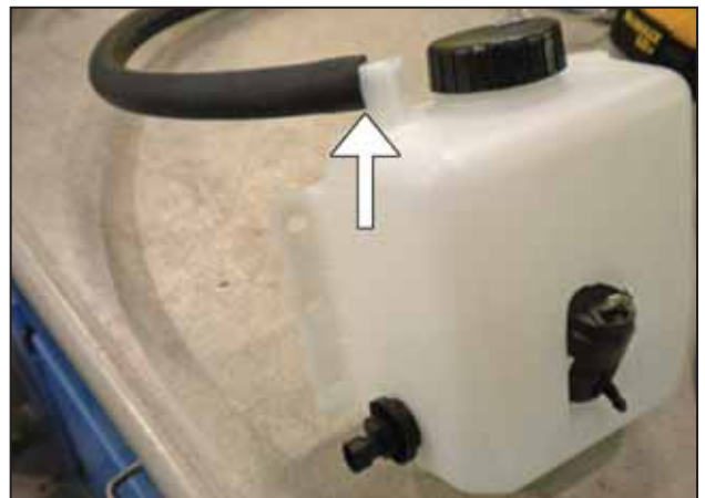
ai. Attach the supplied 5/8" hose to the windshield washer fluid bottle.
