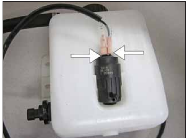
ak. Install the white wire onto the positive terminal of the pump and the black wire onto the negative terminal of the pump
