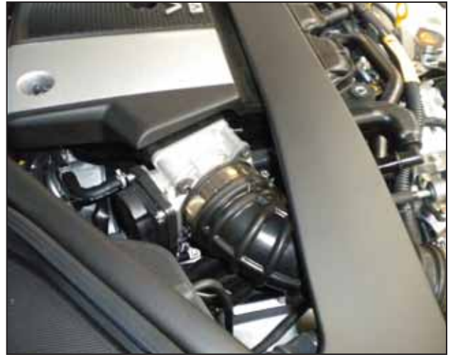
aj. Loosen the hose clamp on the passenger side throttle body.
