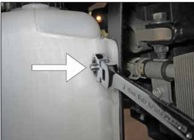
an. Secure the washer bottle to the bracket using the four M6 nuts supplied.
