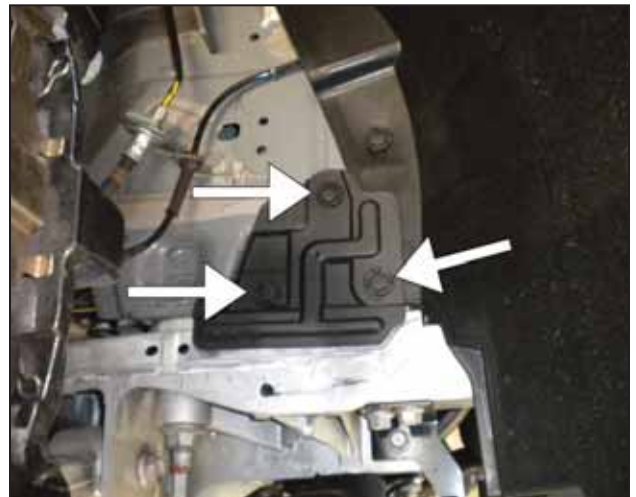
j. Remove the small plastic cover on the passenger side that is exposed once the wheel is removed, 3 clips hold it.
