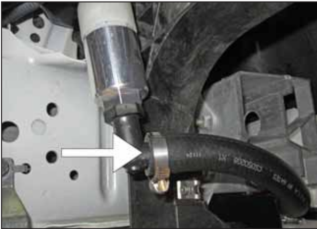
ar. Install the 5/8" hose and secure to the fitting with a hose clamp as shown .
