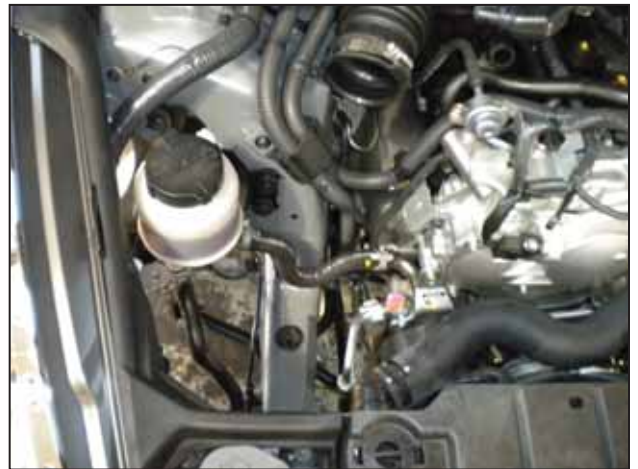
al. Remove the passenger side airbox.
