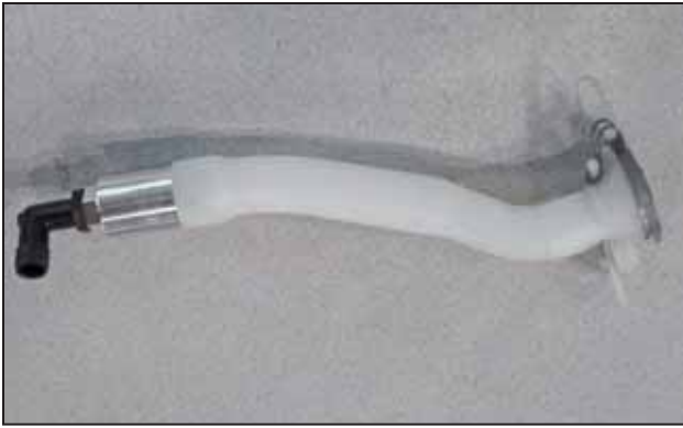
ap. Make sure that the stock o-ring is in place on the filler neck. Attach the adapter onto the filler neck.
