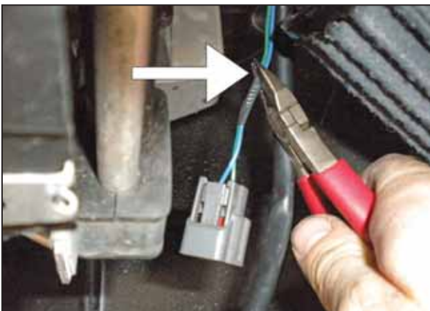
at. Cut the stock pump connector off of the OEM harness leaving some wire on the connector as shown. Do the same for the level sensor.
