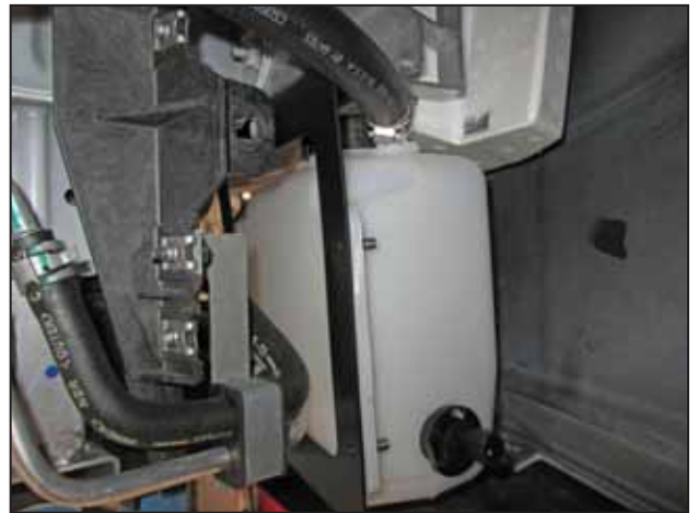
am. Install the washer bottle onto the bracket.
