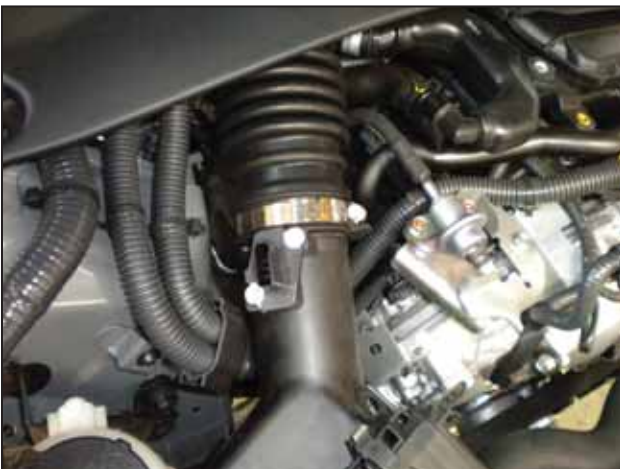
ag. Disconnect the MAF sensor from the passenger side inlet tube.
