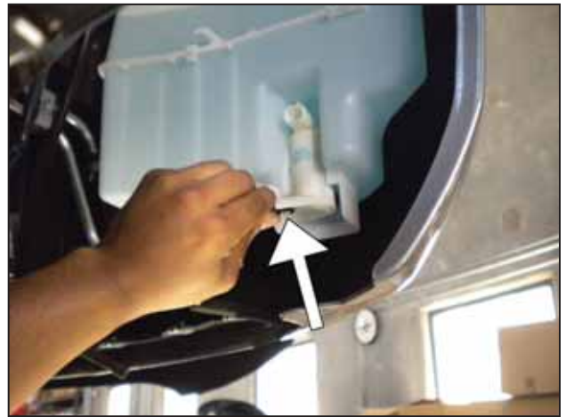
t. Unplug the fluid line from the windshield washer reservoir pump. NOTE: Once the fluid line is disconnected, the pump must be plugged or the windshield washer fluid must be drained into a clean container.
