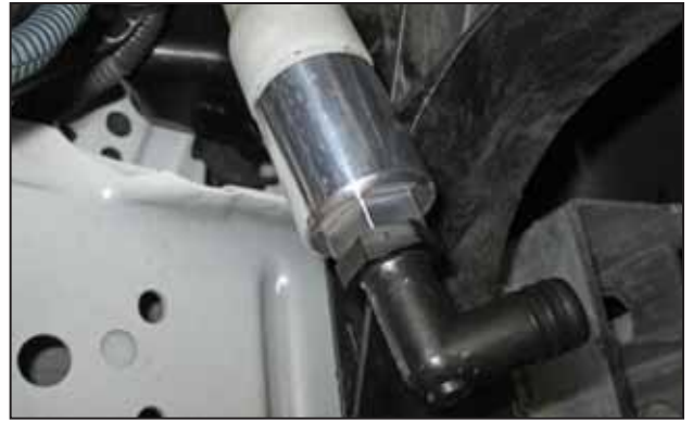
aq. Reinstall the filler neck with the adapter and fitting.
