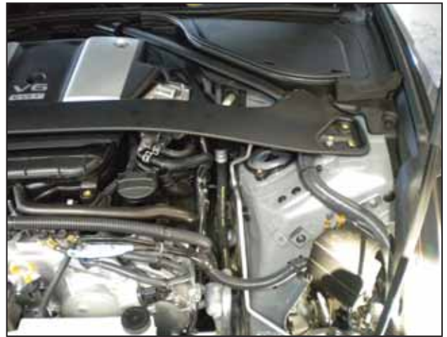
af. Remove the driver side inlet tube.
