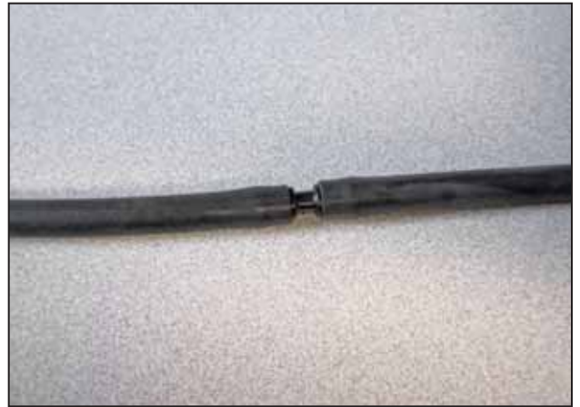
as. Attach the 19" washer fluid hose to the stock washer fluid hose using the supplied hose mender.
