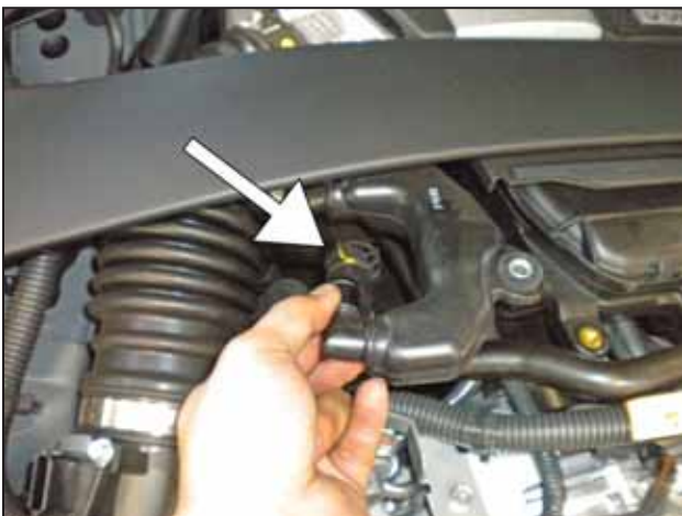
am. Release the hose clamp to remove the PCV hose.
