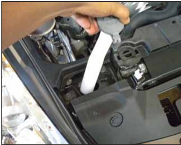
ap. Remove the windshield washer fluid spout.
