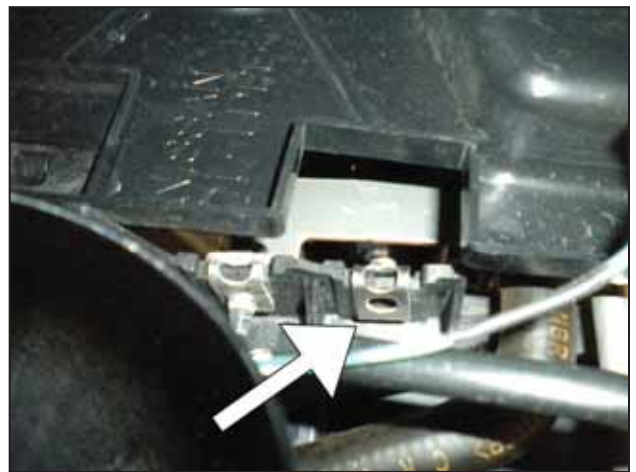
az. Remove the lower windshield washer reservoir clip.
