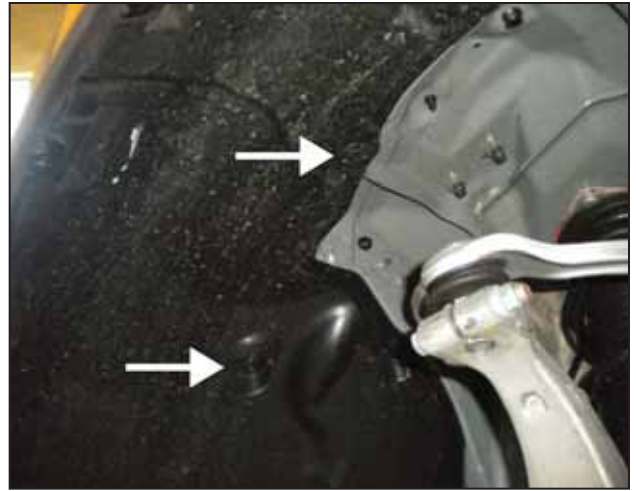
f. Remove the two upper clips securing the fender liner on the driver side.
