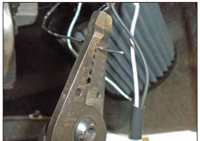
au. Strip the wires on the harness side of the pump.
