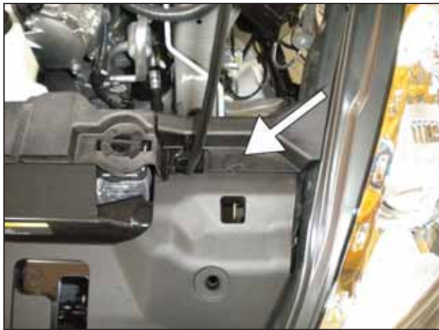
ar. Remove the 1 clip on the driver side as shown.
