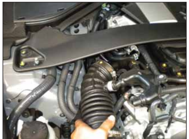
an. Remove the passenger side inlet tube.
