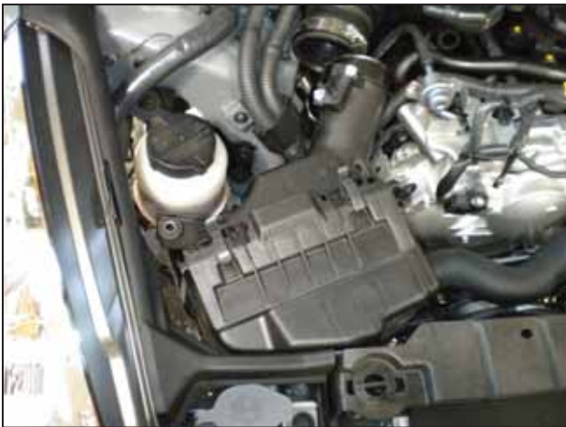
ak. Loosen the hose clamp connecting the passenger side inlet tube to the airbox.
