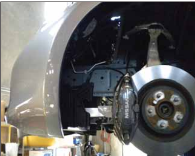
i. Remove the driver side fender liner.
