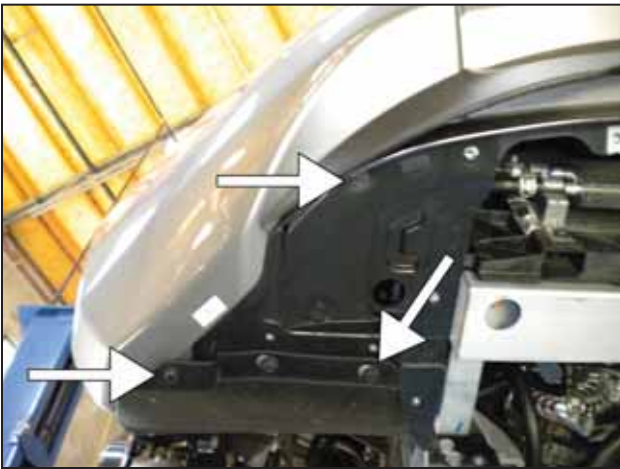
m. Remove the two bolts and one clip securing the fender liner on the passenger side fender.
