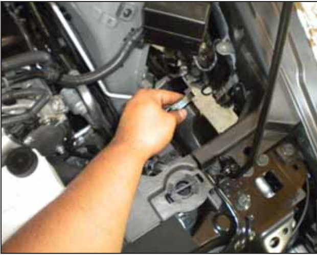
au. Remove the scoop on the driver side.
