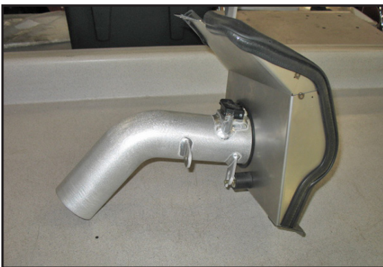
3f. Insert the AEM® intake pipe through the large hole in the heat shield.
