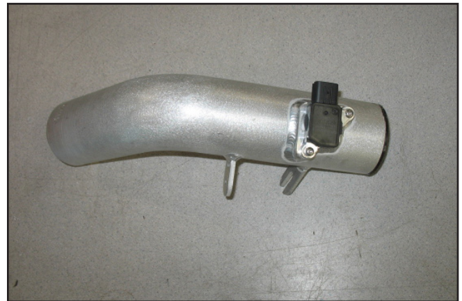
3e. Install the MAF sensor in the AEM® intake pipe with supplied M4 screws.
