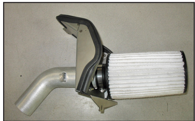
3g. Slide the air filter and #48 hose clamp onto the end of the pipe until the pipe hits the intake pipe stop.
