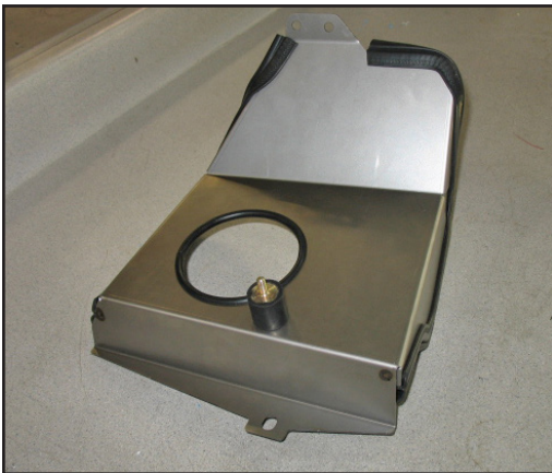
3d. Install a M6 rubber mount on the heat shield and secure with supplied M6 nut.
