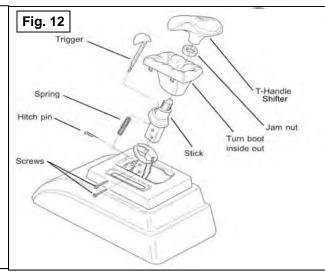
32. Turn the boot right side out and snap the boot into the top plate. Install the T-Handle or knob and jam nut. Tighten the jam nut when the handle/knob is properly oriented. A special jam nut is included with the shifter. It is round with just two flats. The chamfered side goes down. Use a little Loctite on the threads to keep the handle/knob from turning. Check the operation of the shifter.
