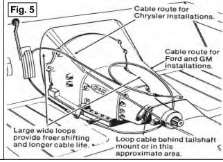
9. Seal the hole where the cable goes through the floorboards to prevent air or water leakage. A putty type sealer can be used. For General Motors vehicles go to Step 10, for Ford vehicles got to Step 15, For Chrysler vehicles go to Step 21.
