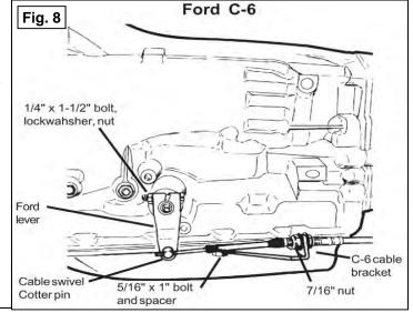
18. Route the shifter cable according to figure 5. Avoid kinks and sharp bends and route the cable away from hot engine or exhaust parts.
