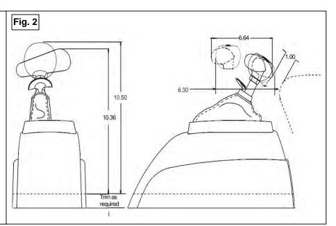
3. Drill four 9/32" mounting holes where marked. Temporarily mount the shifter in place using washers as required to get it level. Do not bend mounting brackets on bottom of shifter. Mark the location for the shifter cable hole, 3" ahead of the left front shifter mounting hole. Drill or cut 1-1/2" diameter cable hole in floorboard.
