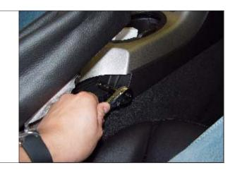
**STEP 16.** Remove passenger side panel and lift up on front center console.
