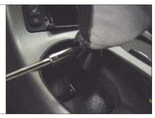
STEP 19. Remove foam and (4) nuts securing rubber.
