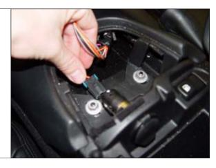
**STEP 6.** Remove panel next to ignition key (temperature sensor) and remove screw.
