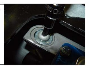
**STEP F.** Remove "L" pin from pin hole and test shifter through each gear.
