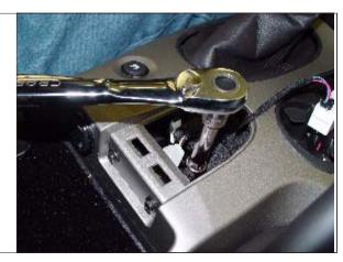
STEP 32. Reinstall (2) screws under passenger airbag panel.
