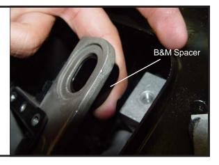
**STEP E.** Place (2) provided washers on top of each spacer and thread bolts securing shifter base to vehicle.
