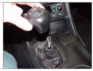
**STEP 42.** Reinstall metal insert into knob and shift pattern indicator.
