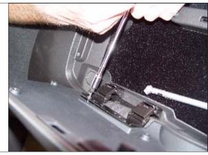
STEP 13. Remove (2) screws under passenger airbag panel.
