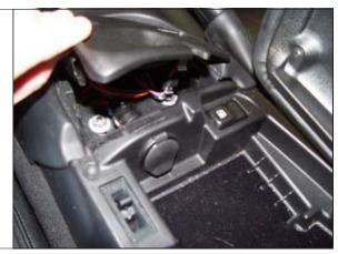
**STEP 5.** Remove (2) retaining nuts and wire connectors.
