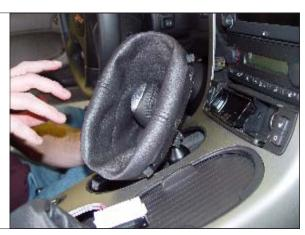
STEP 18. Remove screw securing knob and lift out front center console. Be sure to remove connector wires.
