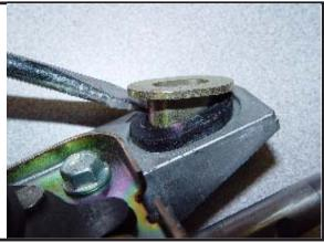
**STEP D.** Install the provided spacers underneath base as shown.
