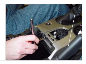
STEP 14. Pull up on sleeve around emergency brake uncovering bolts attaching center console.
