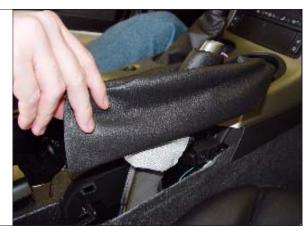
**STEP 15.** Remove (2) bolts holding down front center console.
