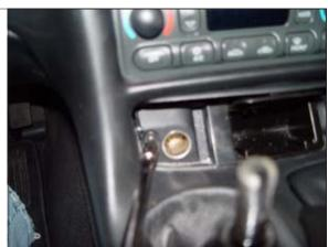
**STEP 38.** Reinstall screw next to ignition key and replace panel.
