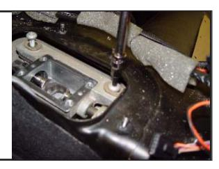
**STEP C.** Remove stock rubber bushings and spacer.
