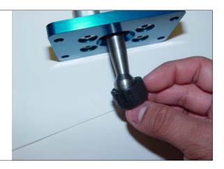
**STEP 23.** Remove old rubber gasket completely and install new gasket.
