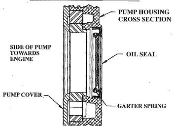
When installing this oil pump take care not to damage the crankshaft oil seal. Before installation lubricate the area of the crankshaft where the oil seal will make contact. Verify that the garter spring is in place. During installation make sure the crankshaft does not damage the oil seal lip or dislodge the garter spring.
