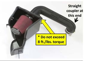
13. Install the barbed fitting  $\implies$  into the brass threaded insert on the FM intake tube as shown.\* Install the provided rubber couplers/clamps onto the FM intake tube and leave loose to allow for rotation.
