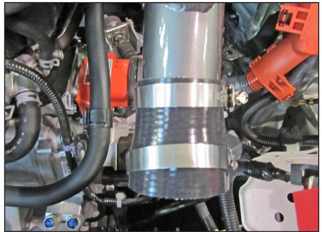
i. Install a reducer coupler (#5-255) onto the end of the upper intake pipe and secure with hose clamp (#9436). Slide hose clamp (9440) onto the open end of the coupler as shown.
