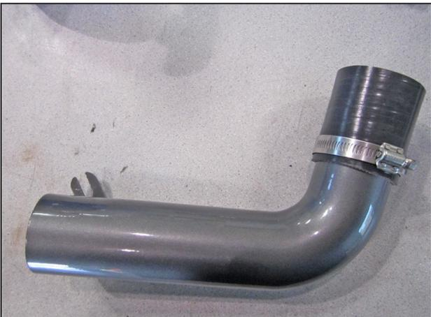
n. Install the 2.75 coupler (#5-250) onto the lower intake pipe and secure with a hose clamp (#9440)
