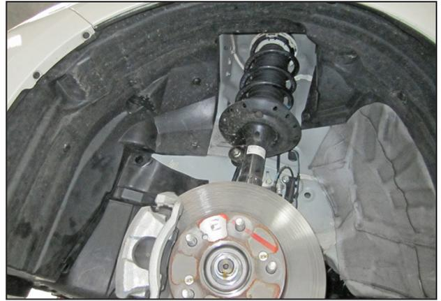
s. Install the fender liner and any hardware that was removed in steps 2l. through 2p.
