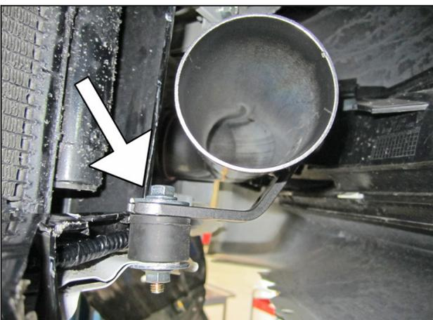
p. Secure the lower intake pipe's bracket to the rubber mount using the supplied washer (#08160) and M6 nut (#44.460.04).
