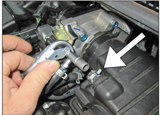
h. Release the PCV clamp on the grommet and pull the PCV tube out.
