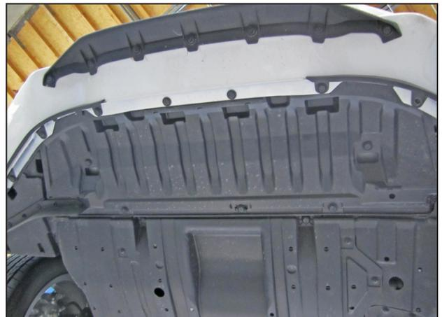
v. Remove the 12 clips and the 2 Phillips head screws securing the belly pan in place, then remove the belly pan from the vehicle.
