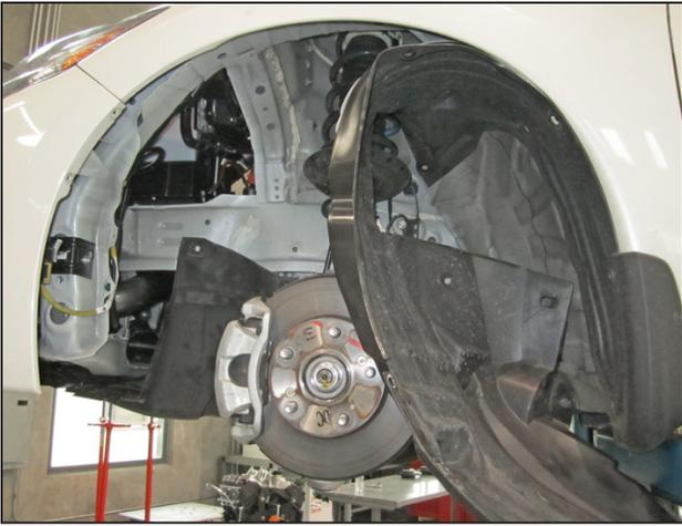
q. Bend the fender liner out of the way to access the inner fender area. Use care so the fender liner is not damaged.
