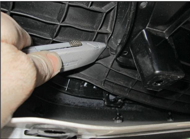
y. Cut the rubber portion of the valence at the narrow section of the valence near the bottom.
