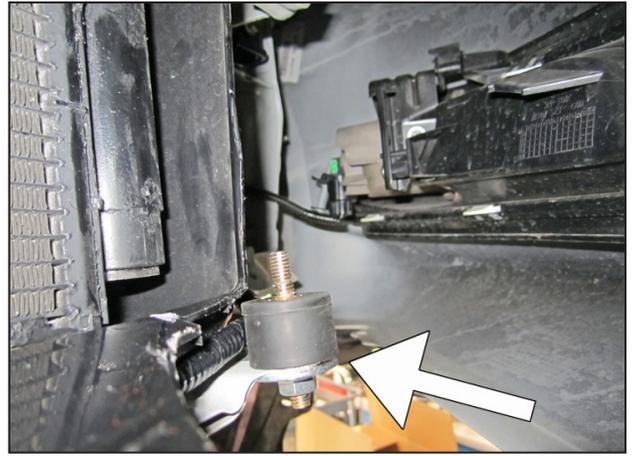
m. Install the lower rubber mount (#1228598) to the specified location and secure with the provided washer (#08160) and M6 nut (#44.460.04).
