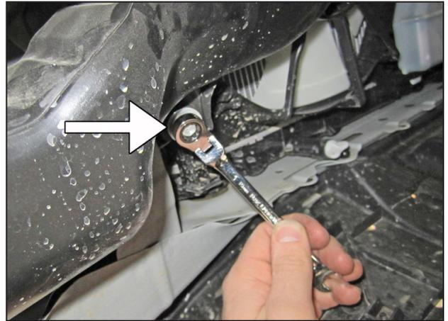
t. Remove the remaining 10mm bolt securing the resonator.
