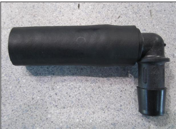
d. Insert the 90° fitting (#8-157) into the 1/2" hose (#5-5003) as shown.
