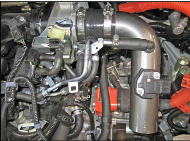
h. Install the upper intake pipe as shown. Re-install PCV hose.
