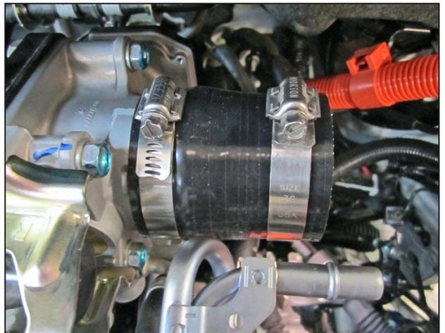
c. Install the reducer coupler and secure to the throttle body with hose clamp (#9440). Slide hose clamp (#9436) onto the open end of the coupler.
