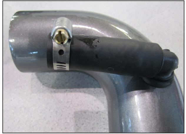
g. Slide hose clamp (4093-5) onto the hose as shown.
