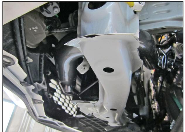
o. Install the lower intake pipe and route as shown. Secure the end with the coupler to the middle intake pipe while also aligning the intake pipe's bracket with the rubber mount installed in step 3m.
