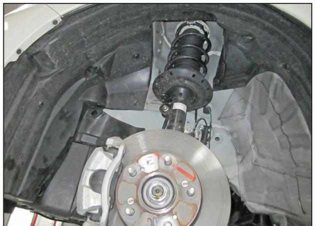
p. Remove the 9 clips securing the fender liner to the fender well.
