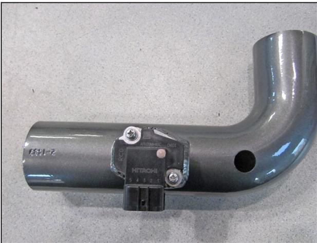
b. Install the mass air flow sensor in the upper intake pipe using the stock MAF screws.
