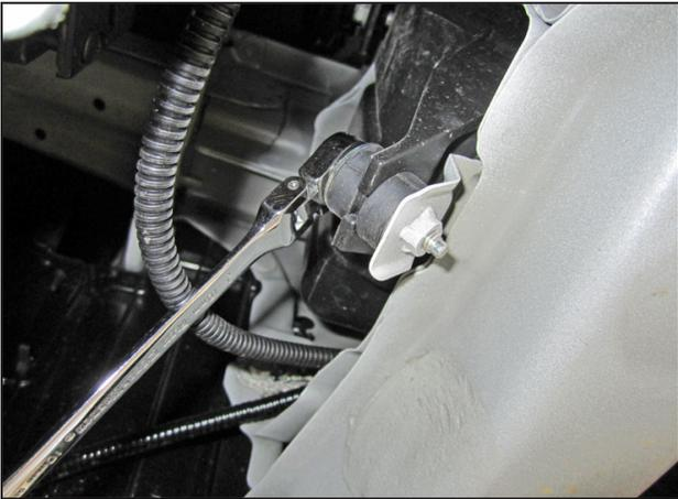
s. Remove the lower 10mm bolt securing the resonator.
