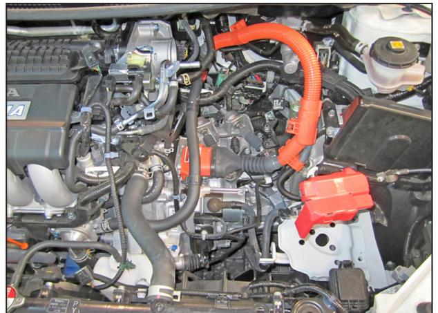
j. Remove the stock air box system from the vehicle.
