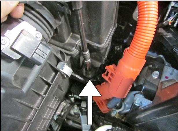
g. Remove the 10mm bolt from the right side of the air box.
