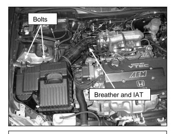
a. Loosen the two bolts holding the factory air box to the inner fender. Remove the cam cover breather and intake air temp sensor (IAT). Remove the factory air box.
