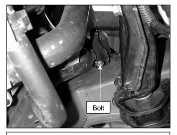
e. Loosen the bolt holding the lower air tube bracket to the frame rail, and remove it.
