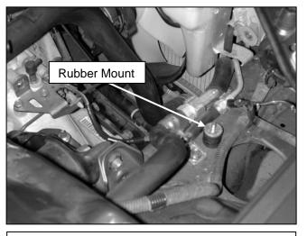
e. Install the supplied rubber mount in the threaded hole in the frame rail as shown.
