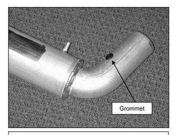
f. Install the included rubber grommet in the intake pipe as shown.
