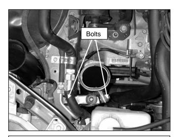
b. Loosen the bolts holding the lower air tube to the frame rail.
