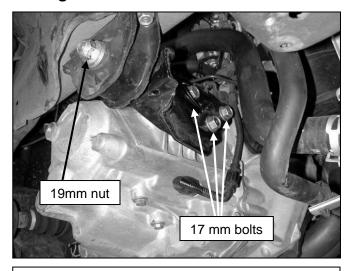
a. Using a 19mm socket, remove the engine mount nut, then loosen the three bolts with a 17mm wrench, and remove the mount.
