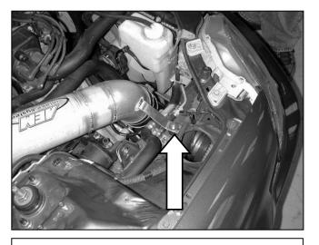
h. Using the included washer and nylock nut, secure the intake pipe bracket to the rubber mount as shown.
