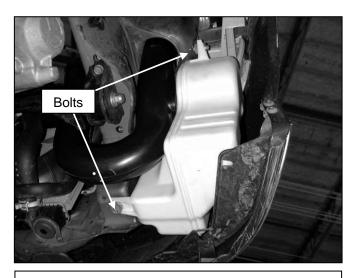
d. Loosen the two bolts holding the resonator box to the inner fender; remove it along with the lower air tube.
