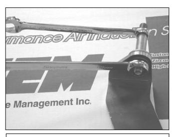
c. Install the factory mounting stud from step 3b on the supplied engine mount bracket, using the provided nylock nut and washer.
