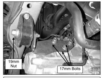
d. Using the supplied bolts and the factory washers, install the AEM® engine mount on the transmission; torque the bolts to 61 ft-lb. Then replace the factory washer and nut on the mounting stud.
