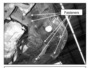
c. Remove the fasteners securing the fender liner and splash shield. Remove the fender line and splash shield to access the fender well.
