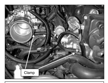
d. Install the supplied 5/15" hose on the coolant outlets using the factory clamps as shown.
