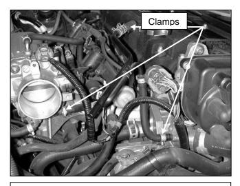
c. Remove the clamps securing the cam cover breather tube and coolant circulation tube, and remove it (Some coolant will come from the manifold and head).
