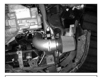
i. Install the AEM<sup>®</sup> air filter onto the short leg of the lower intake pipe. Then attach the lower pipe assembly to the upper intake pipe using the supplied coupler and hose clamps. Position the assembly so the air filter has adequate clearance.
