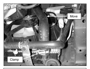
b. CAUTION: Ensure the engine is completely cool before removing the coolant hose, or hot coolant will escape from the cooling system and cause injury or damage.
