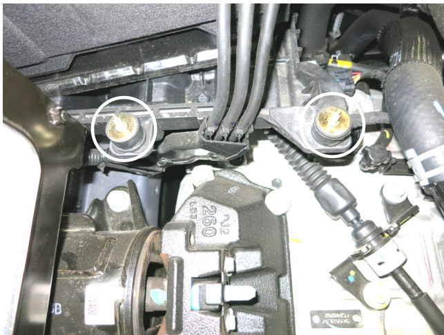
d. Install the two rubber mounts into to vehicle.
