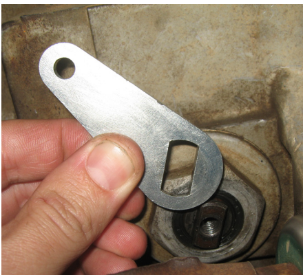
Figure 30: New Transfer Case Shift Lever Orientation
