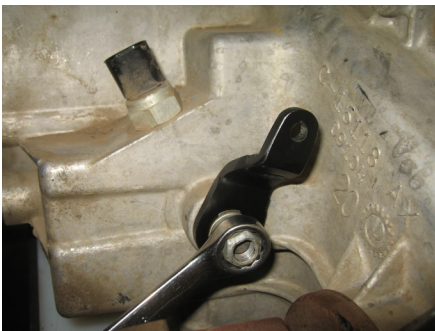
Figure 29: New Transfer Case Shift Lever Orientation
