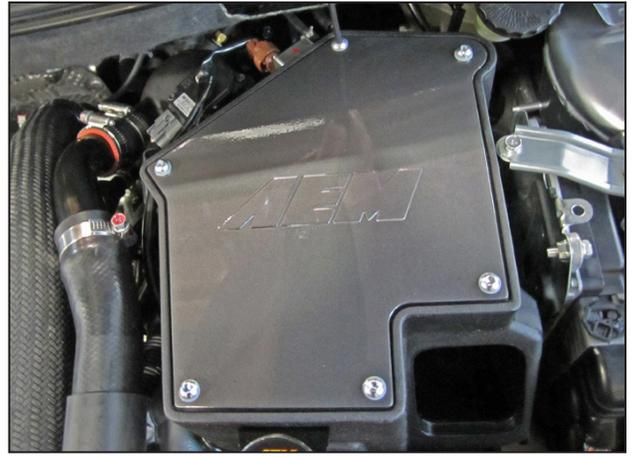
ae. Install the aluminum heat shield lid onto the air box top. Secure the heat shield lid in place using the 6 plastic washers (1-3001) and 6 button-head bolts (1-112). Install all the hardware before completely tightening. Once the heat shield lid is properly aligned, fully tightening the hardware by starting at the back of the air box and moving in a clockwise direction.
