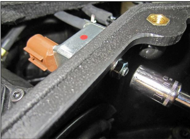
ab. Mount the wastegate solenoid to the hole on the back side of the AEM® air box using the stock 10mm nut. Align the solenoid's small tab with the dimple next to the mounting hole and fully tighten the nut to secure the solenoid to the air box.
