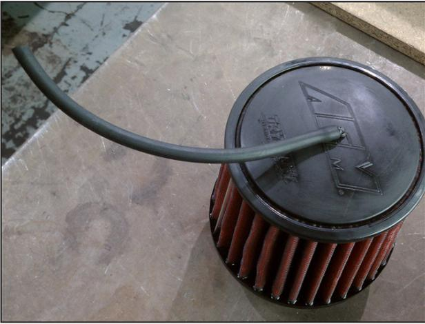
v. Install the provided elbow fitting (8-152) into the AEM® air filter's top (21-2031D-H). Install the provided hose (5-3009) onto the end of the elbow port as shown.
