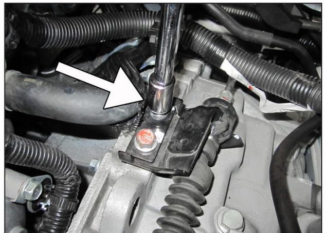
v. Locate the shift cable bracket on top of the transaxle case. Remove the specified 12mm bolt securing the shift cable bracket. This bolt will be reused in a later step during the installation of the AEM® intake system.
