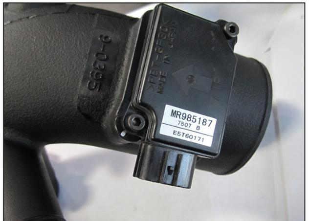
e. Mount the stock MAF sensor onto the upper intake tube (9-0395) using the provided M4 Allen bolts.
