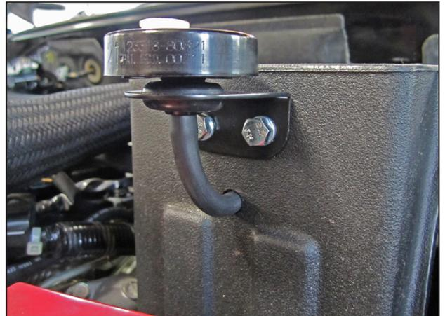
y. Locate the hose (5-3009) attached to the AEM® air filter and route the hose through the hole in the air box below the AEM® filter minder gauge. Connect the hose to the gauge's outlet. Trim any excess hose.
