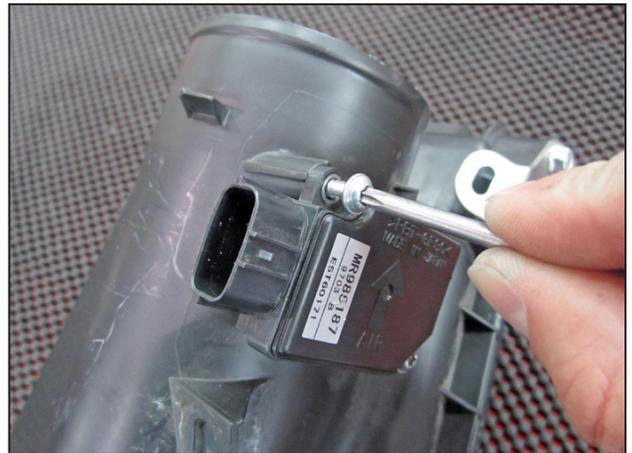
p. Remove the MAF sensor from the air box outlet tube. The MAF sensor will be reused in a later step during the installation of the AEM® intake system.
