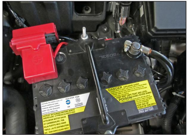
ag. Reconnect the negative battery cable to the battery.
