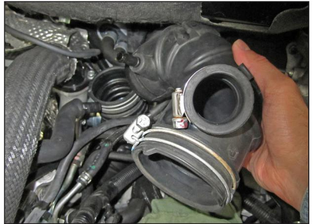
t. Unfasten the middle hose clamp and remove the upper intake tube from the lower tube.
