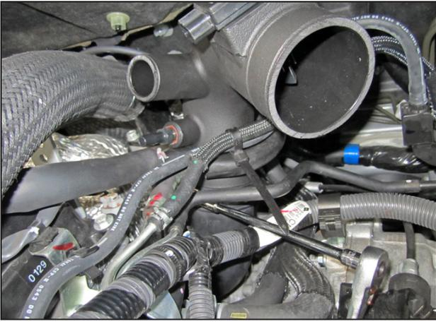
l. Install the upper intake tube onto the large end of the elbow coupler as shown. Tighten the upper #48 hose clamp, but not completely so the intake tube can rotate slightly.
