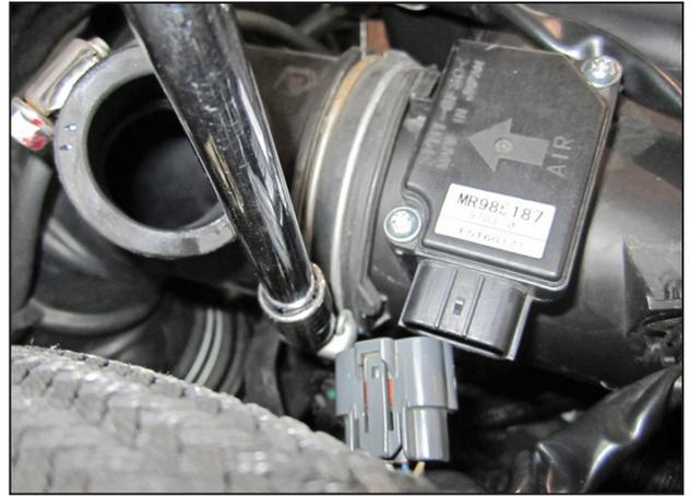
l. Locate the hose clamp securing the air box outlet to the intake tube and unfasten.
