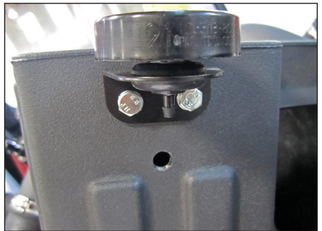
i. Insert the filter minder gauge onto the filter minder bracket (32-3017). Attach the filter gauge assembly onto the air box using the two M6 hex bolts (1-2065) and two split washers (1-3025) as shown.
