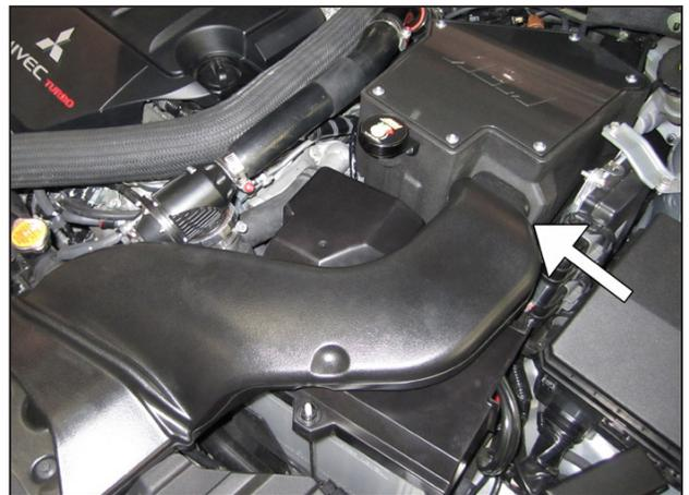
ai. Install the stock intake scoop into the matching inlet of the AEM® air box and over the battery cover.
