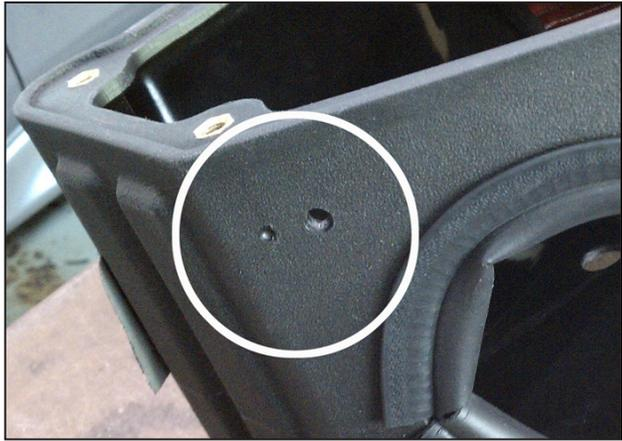
aa. Note the small alignment dimple next to the wastegate solenoid mounting hole on the AEM® air box. When the wastegate solenoid is mounted to the air box ensure the alignment tab (Pointed out in Step 3z) aligns in the dimple.
