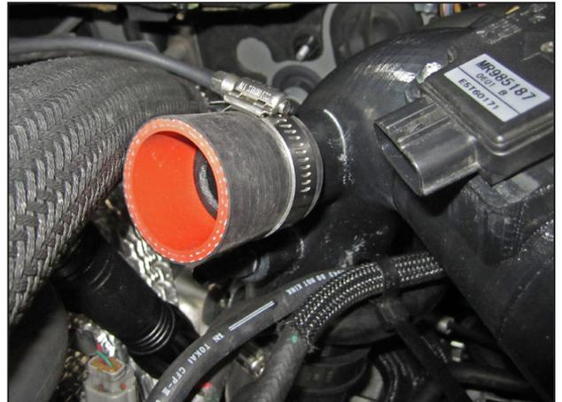
s. Install the silicone hose (5-1055) onto the AEM® intake tube. Attach the silicone hose about 1/3 of the way onto the turbo bypass port. Secure in place with a #28 hose clamp (103-BLO-2820).
