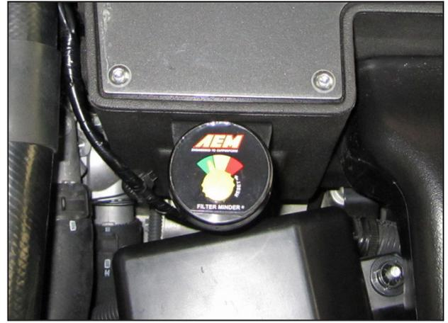
ak. Ensure the needle on the AEM® filter minder gauge is set to the “Green” section on the indicator.
