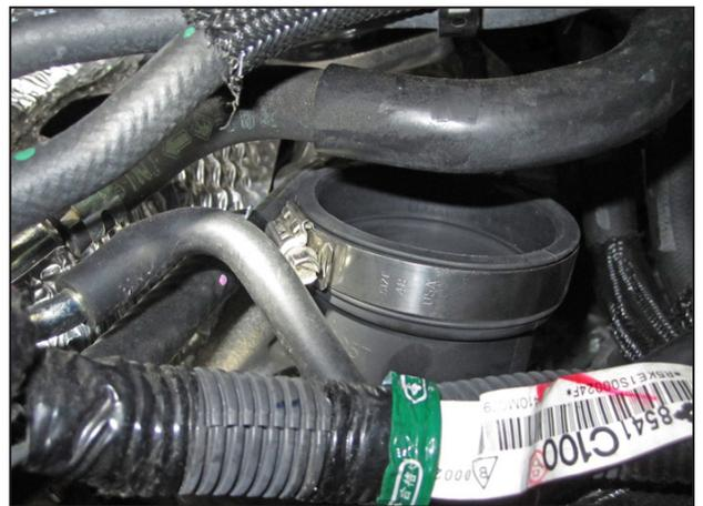
k. Install the elbow coupler (5-1057) to the turbocharger compressor inlet as shown. Tighten the smaller #36 hose clamp slightly, so the elbow coupler can still rotate on the compressor inlet. Use two 1/4" drive extensions and a drive u-joint to ease installation.
