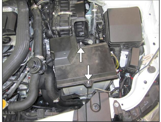
b. The vehicle's battery is located under the stock intake scoop. Remove the plastic retaining nuts and battery cover to access the battery.
