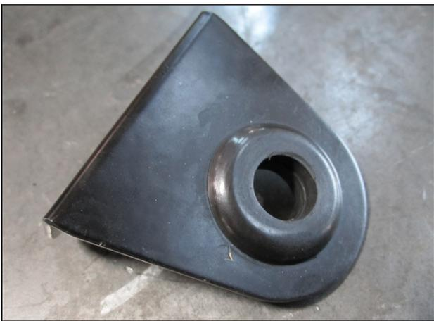
h. Install the rubber grommet (784634) in the filter minder bracket (32-3017) as shown.
