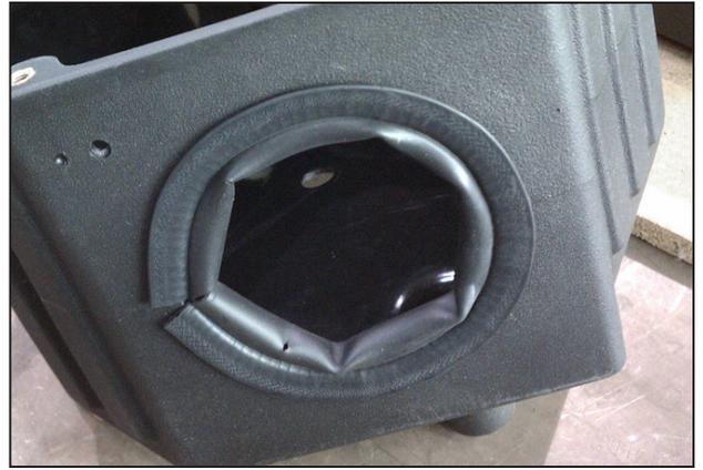
g. Install the edge trim (8-4015) around the large outlet in the air box as shown. Trim the edge trim if necessary.
