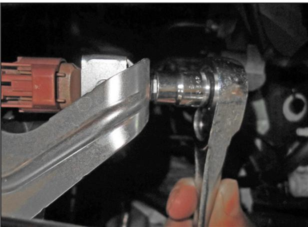
m. Remove the 10mm nut that holds the turbocharger wastegate solenoid to its metal bracket on the air box. The nut will be reused during the installation of the AEM® intake system.
