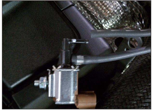
r. Completely remove the small black hose from the upper solenoid port.
