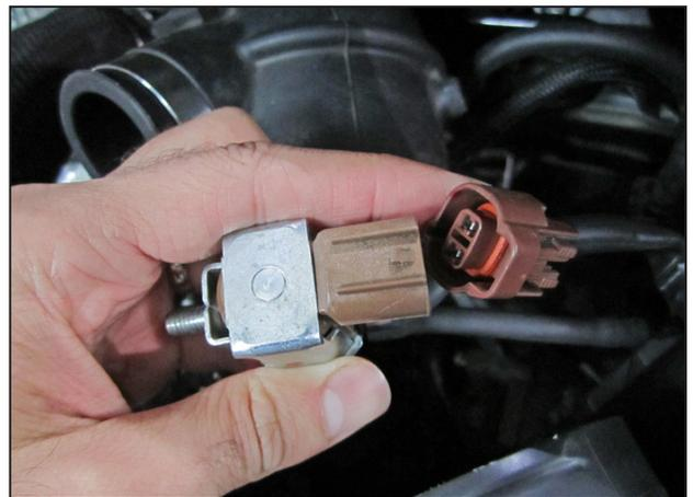
n. Disconnect the wastegate solenoid from its wiring harness. Disengage the long black solenoid hose from the 2 rubber retainers along the side of the intake tube, but leave connected to the solenoid. Set the solenoid aside in a safe area.
