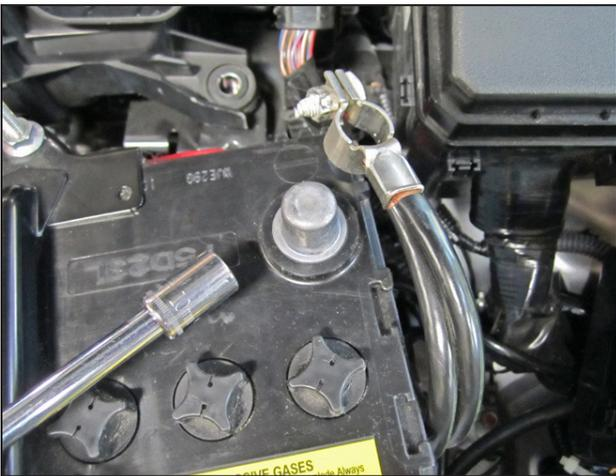
c. Disconnect the negative battery cable.
