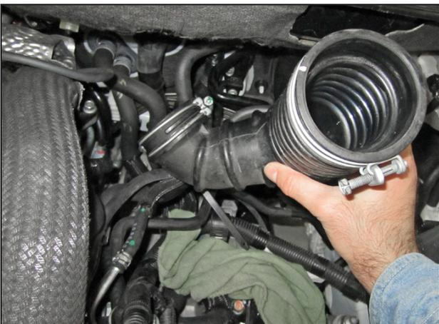
u. Unfasten the lower hose clamp at the turbo inlet and remove the lower intake tube from the turbocharger.
