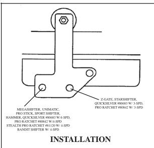
**Note:** Be careful. Select the correct hole for your shifter. Wrong hole **will** destroy the cable, shifter and/or transmission in **one** shift! (GM trans. only)
