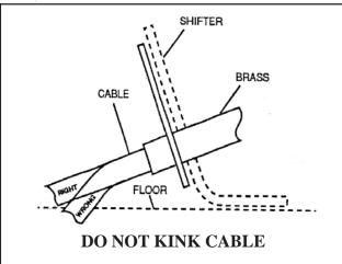
**Note:** Do not kink cable anywhere along it's length. If cable has a kink, it will lock up. Cable should be kept straight for 2 inches on each end where it leaves the brass. Any of the above **will** destroy the cable, shifter and/or transmission in **one** shift!
