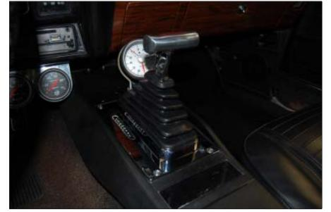
steering column lock will work and will allow the key to be removed. The cable should also be secured inside of the console out of the way. After wiring the cable in this position, check to see that the steering column lock works correctly, and that you can remove the key. WARNING: With the interlock disabled in this manner, it is possible to lock the steering column at any time, so be careful not to turn the key to the "LOCK" position while the car is moving.
