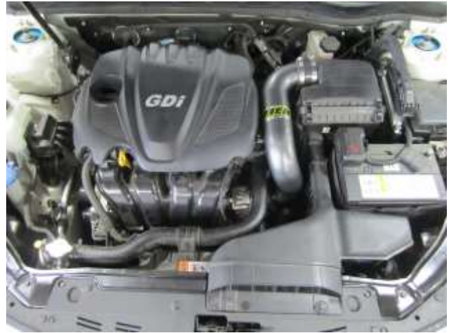
AEM Intake Installed.
