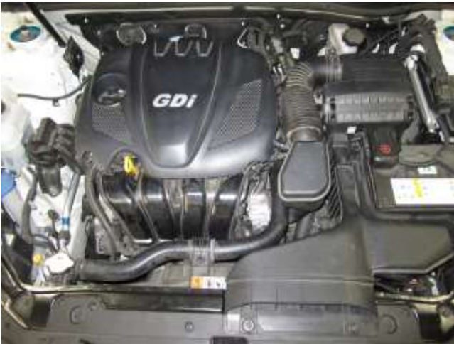
Stock Intake Installed.
