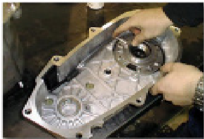
(Fig. 6A) Case Half Pre-assembly
