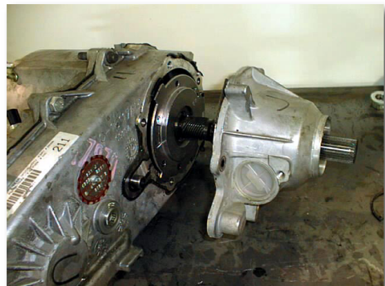
(Fig. 8) Rear Tailhousing Removal
