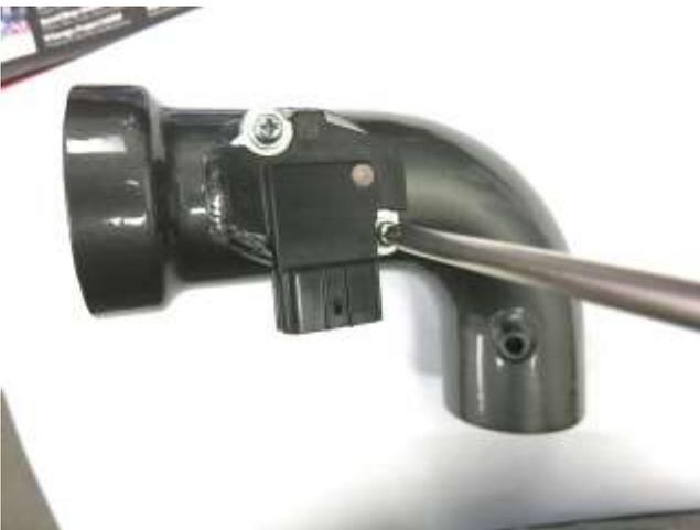
a. Use the stock screws removed in step 2f to fasten the MAF sensor into the AEM tube.
