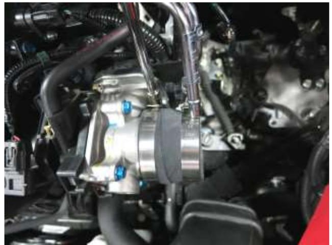
b. Install the transition coupler(08476) and fasten the hose clamp(AEM-9440) over the throttle. Slide loose hose clamp(AEM-9436) over the other coupler end.
