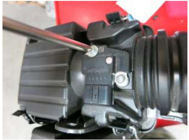
f. Use a phillips screwdriver to remove the MAF sensor. Set aside the stock screws for use with the AEM tube.
