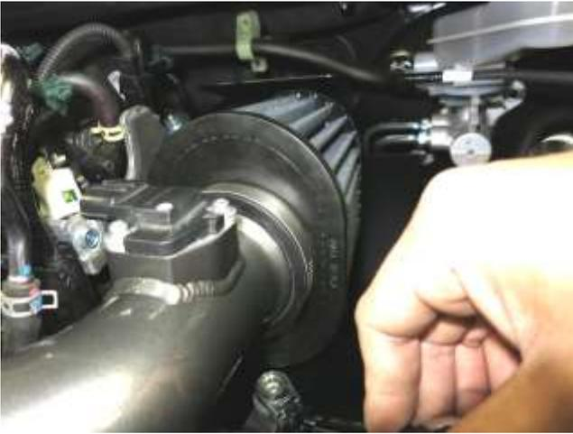
i. Fasten the lower bracket down using the nut(AEM-444.06.04) and washer(08160) provided.
