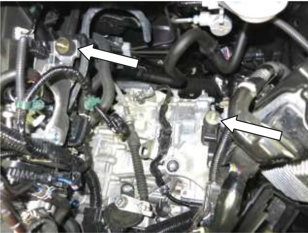
c. Install the two rubber mounts(AEM-1228598) onto the stock airbox mounting locations as indicated.
