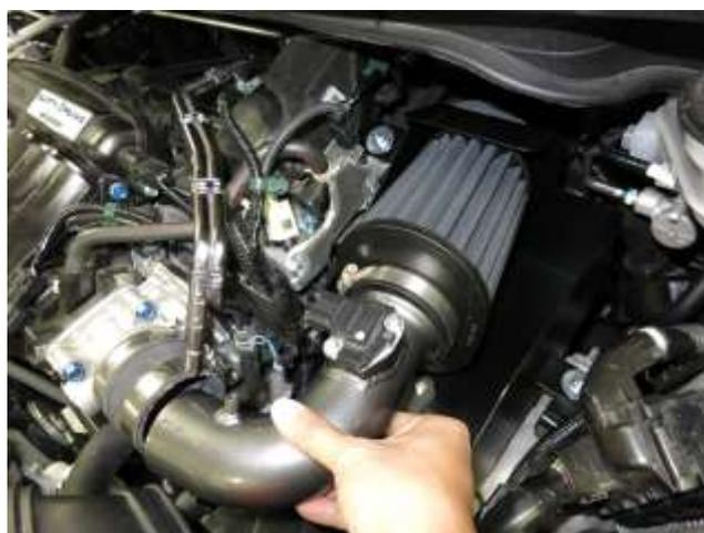
g. Insert the intake tube into the coupler and align the lower rubber mount to the lower bracket.
