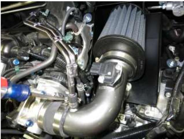
j. Adjust tube position if needed and fasten the hose clamp on the coupler.
