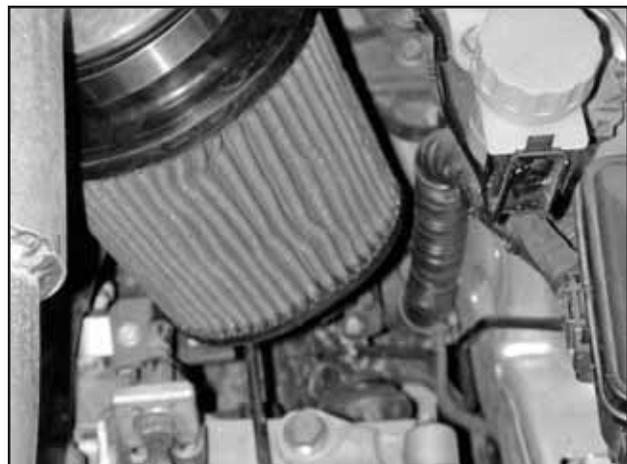
i. Install the AEM® filter on to the end of the inlet tube. Push the filter over the inlet pipe until the stop in the filter is reached and install #56 hose clamp to secure the filter onto the inlet pipe. Once fitment is checked, tighten the hose clamp after this is done.
