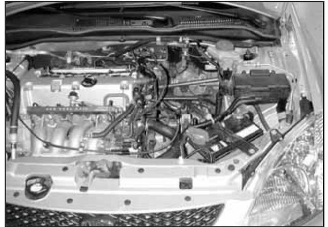
l. Factory air box system removed.
