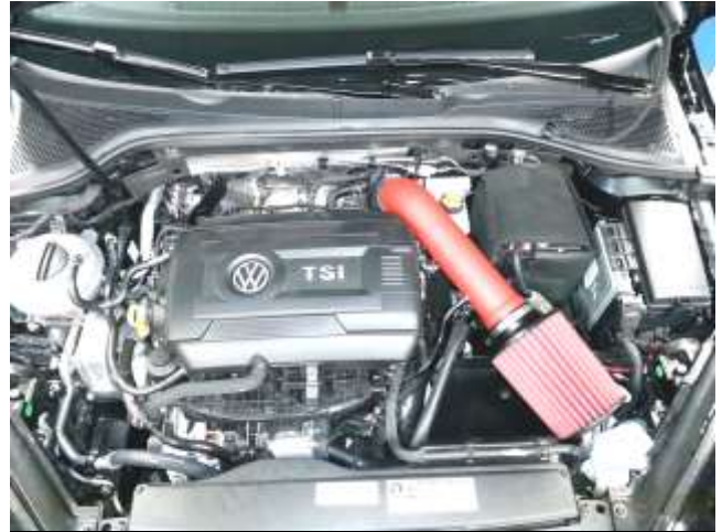
AEM INTAKE INSTALLED
