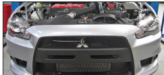
Stock Intercooler System Installed.
