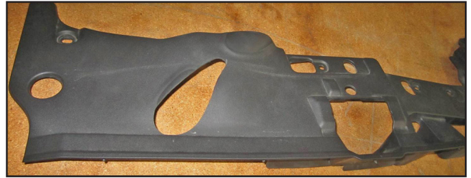
n. The front plastic cover will have to be modified to clear the new AEM charge pipe. Tape down cut-out template on indicated edges as shown and etch onto plastic cover using a razor blade. Use a hand-held rotary tool to cut out shape specified.
