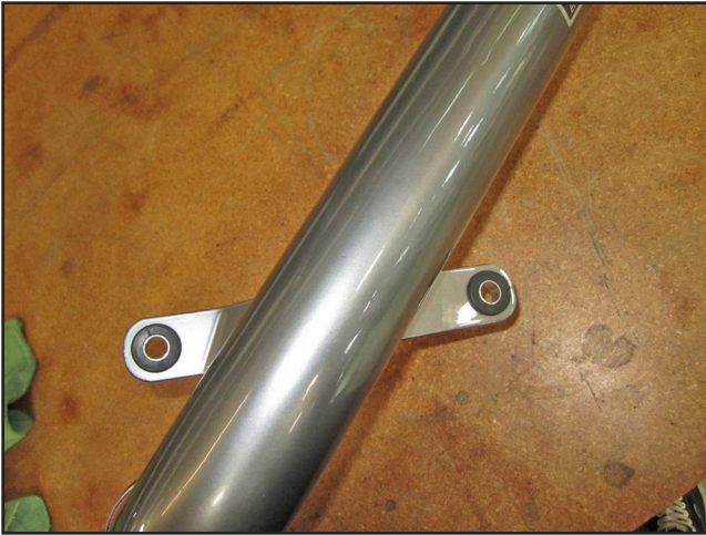
k. For upper charge pipe(2-1483), install rubber grommets and sleeves removed in Step 2i into brackets as shown.
