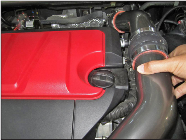
m. Rotate and adjust upper pipe (2-1482) to line up with previously installed charge pipe(2-1483). Check and adjust for clearance along engine cover and valve cover breather hose.
