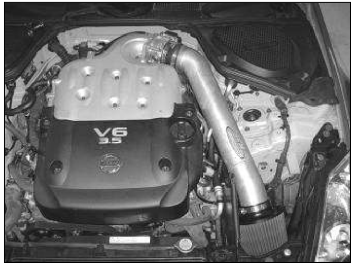
AEM® intake system installed
