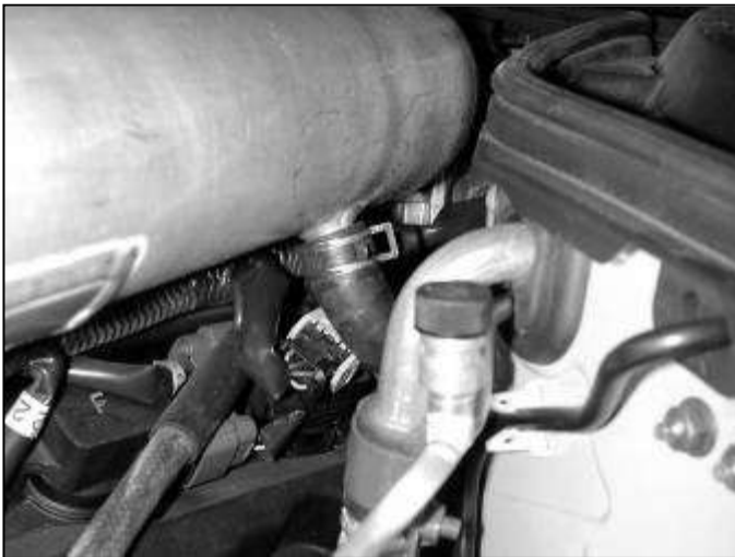
n. Reattach the crankcase breather hose to the inlet pipe. Secure with the factory spring clamp.
