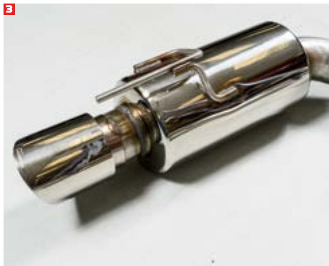
3 The Hooker BlackHeart cat-back includes polished mufflers and double-wall, 4-inch stainless steel tips laser etched with the Hooker logo.
