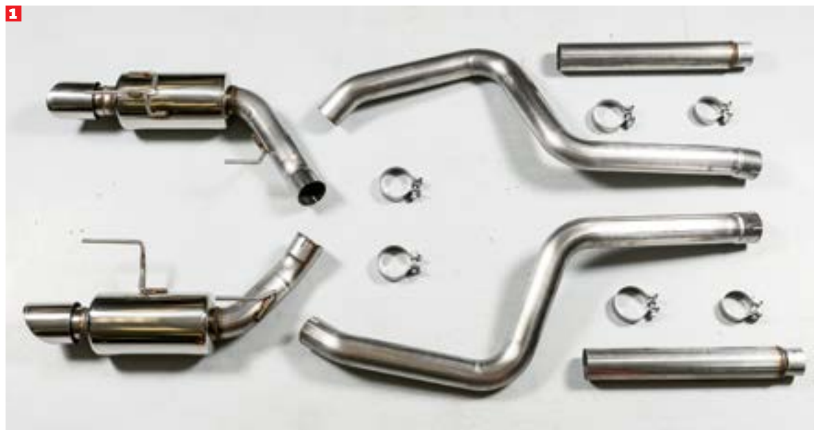
1 The Hooker BlackHeart cat-back exhaust for 2005-2009 Mustang GTs features 304 stainless steel construction, straight-through mufflers and is 8 pounds lighter than the factory system.
