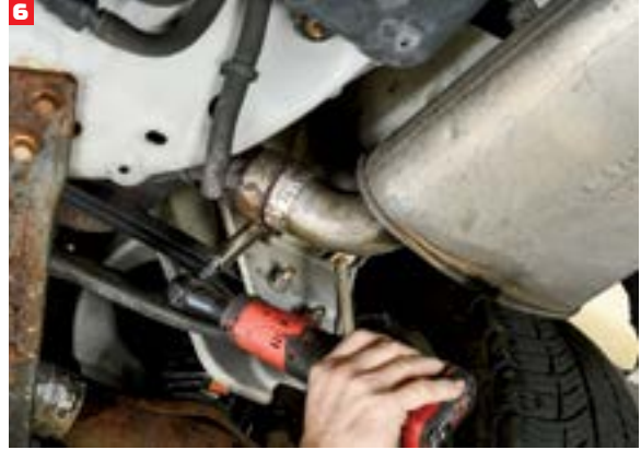
Then he loosened the OEM muffler's clamp from the over-axle pipe.
