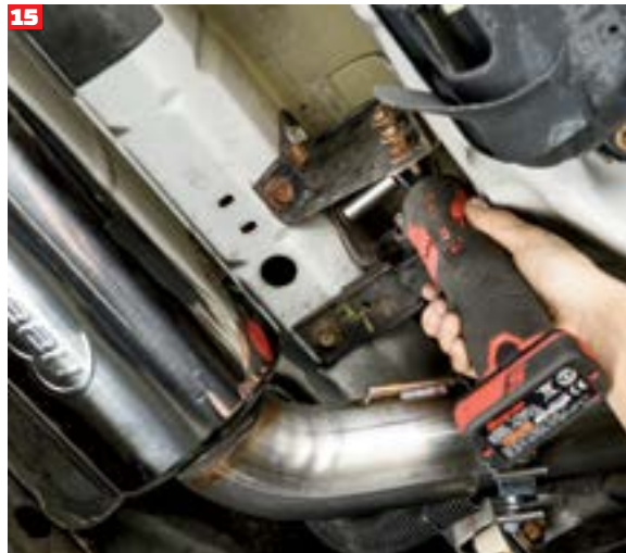
15 Since the Hooker mufflers are considerably smaller than their OEM counterparts, accessing the hanger bracket fasteners was much easier.
