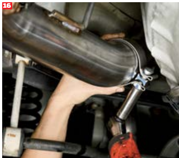
16 With the mufflers in place, Weathers loosely installed the clamps.
