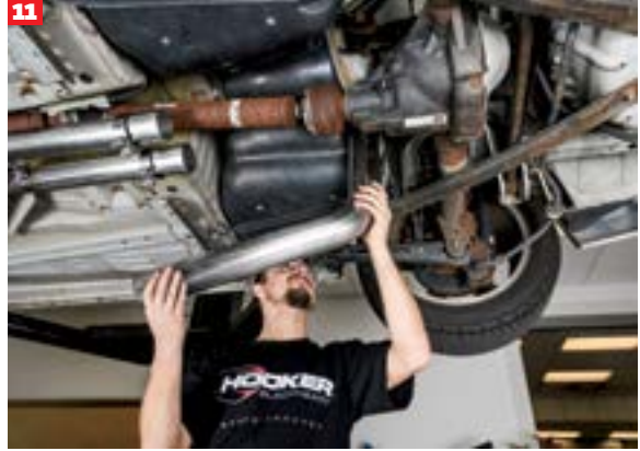
Then he snaked the 3-inch over-axle pipes into position.
