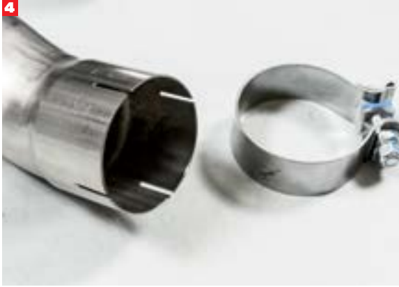
To ease installation and clearance adjustment, the cat-back features leak-free slip fit joints and high-quality band clamps.
