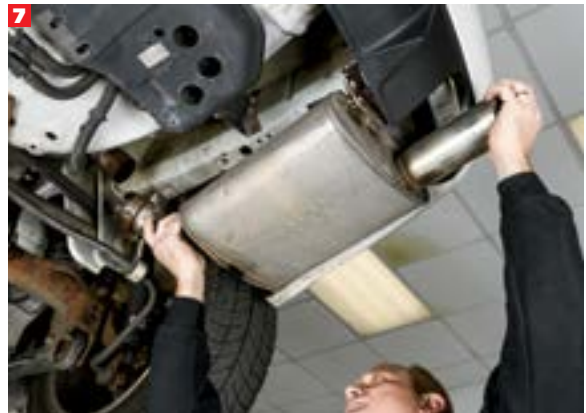
After a little wiggling (some spray lube helps), we removed the OEM mufflers.
