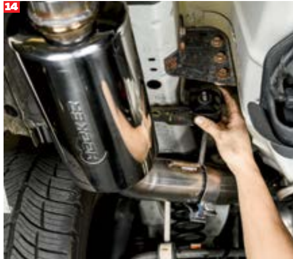
14 He reused the OEM hanger brackets and isolators with the Hooker cat-back system.
