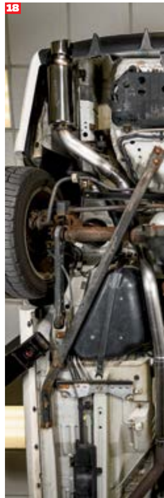
15 Since the Hooker mufflers are considerably smaller than their OEM counterparts, accessing the hanger bracket fasteners was much easier.
