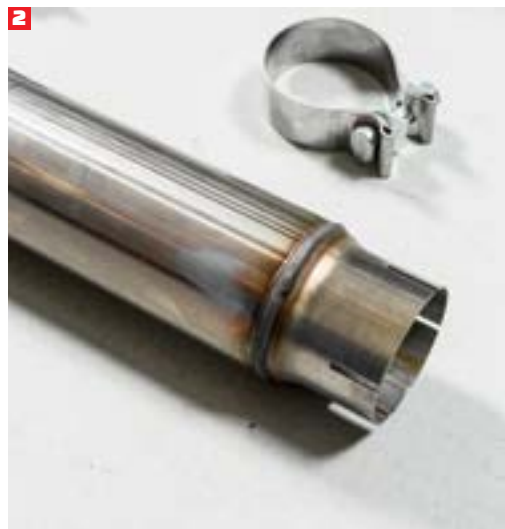
2 The 3-inch tubing of the cat-back system connects to the factory H-pipe with a slip fit joint and a stainless steel band clamp.
