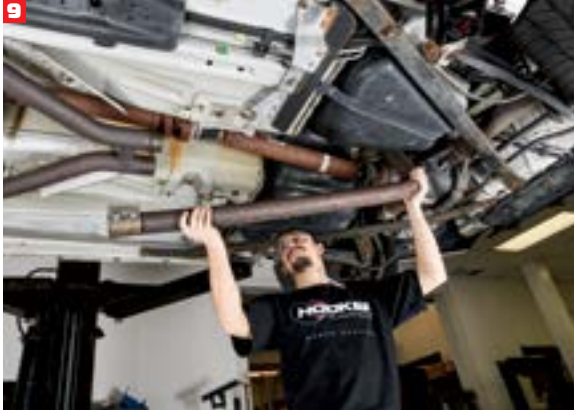
With the clamps loose, Weathers slid the OEM over-axle pipes backwards and removed the pipes from the chassis.
