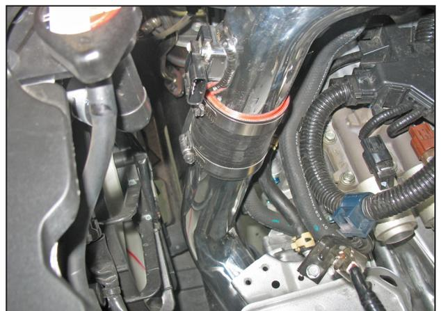
o. Align the lower intake pipe with the upper intake pipe and orient as shown. Insert the lower intake pipe into the upper intake pipe's coupler and loosely secure the #9440 hose clamp.
