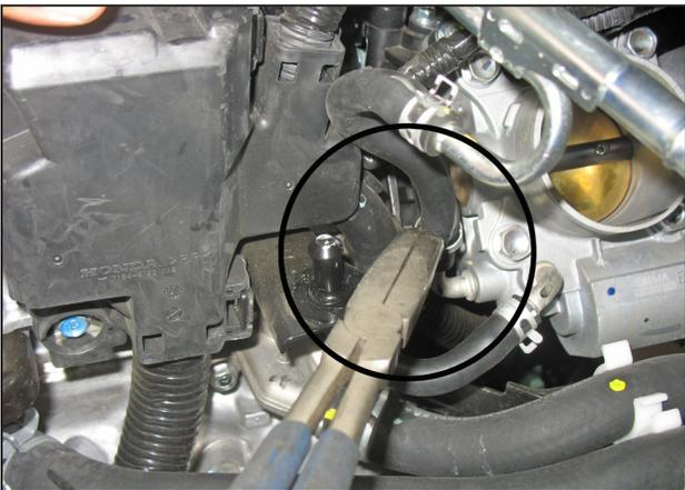
m. **CAUTION: Ensure the engine is completely cool before removing the coolant hose, or hot coolant will escape from the cooling system and cause injury or damage. Be sure to capture any lost coolant in a clean container.** Remove the coolant hose connected to the throttle body (This hose is connected to the hard line that is attached to the PCV hard-line).
