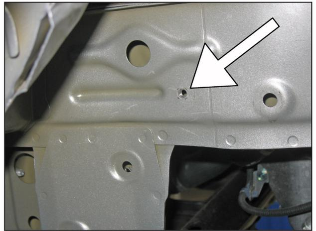
m. Install the second rubber mount in the thread-hole exposed in step 2u.
