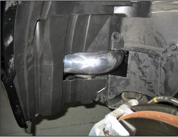
t. Trim the fender liner to clear the intake pipe. Install the fender liner and any hardware that was removed during steps 2r and 2s.
