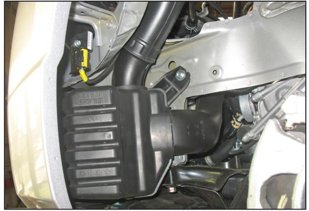
t. Remove the two bolts securing the lower resonator to the vehicle.
