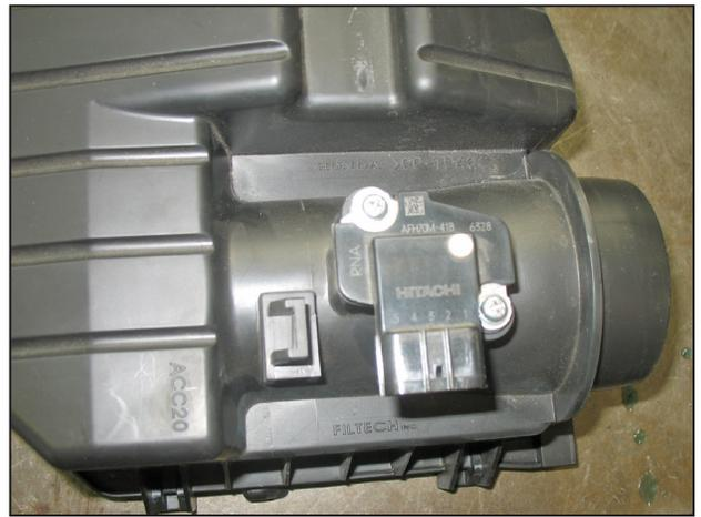
v. Remove the mass air flow (MAF) sensor from the lid of the stock air box.
