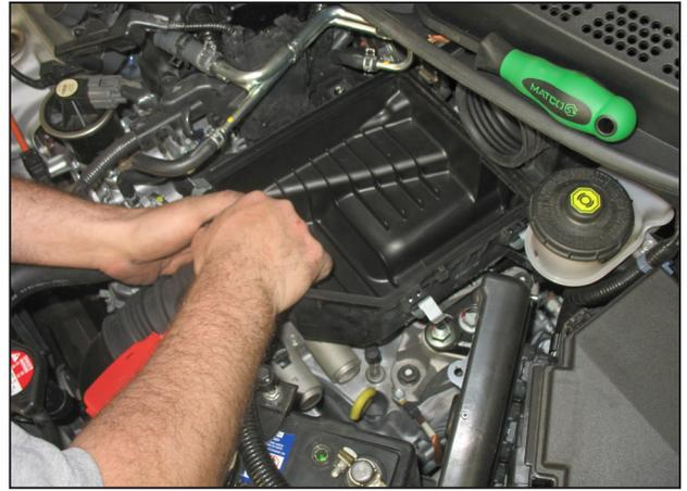
l. Disconnect the rubber inlet duct from the front of the air box, then remove the air box from the vehicle. Remove the inlet tube from the throttle body.
