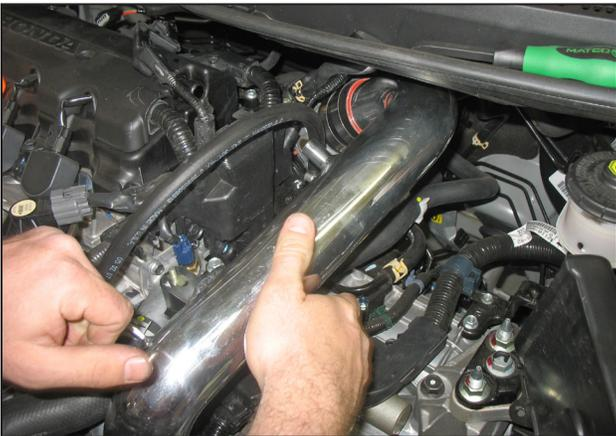
h. Insert the upper intake pipe into the silicone hose installed on the throttle body.
