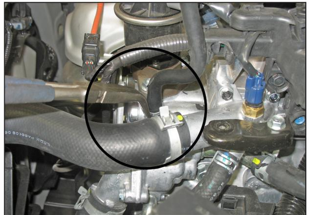
n. Remove the other side of the coolant line connected to the engine.
