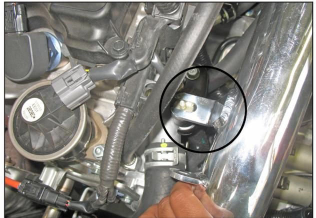
i. Align the bracket with the rubber mount installed in step 3d.
