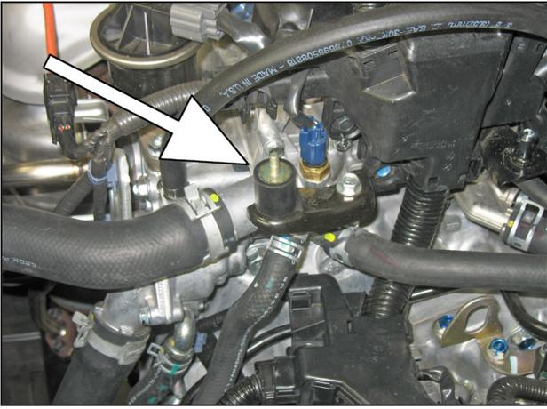
d. Thread one rubber mount into the stock mounting location.
