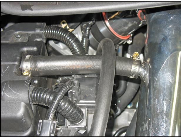
l. Install the 5/8" hose onto the upper intake pipe nipple and the valve cover nipple. Secure each end with a 1 1/16" hose clamp.
