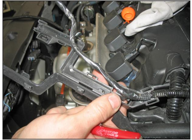
q. Remove the hard plastic casing on the MAF sensor harness to expose the wires.
