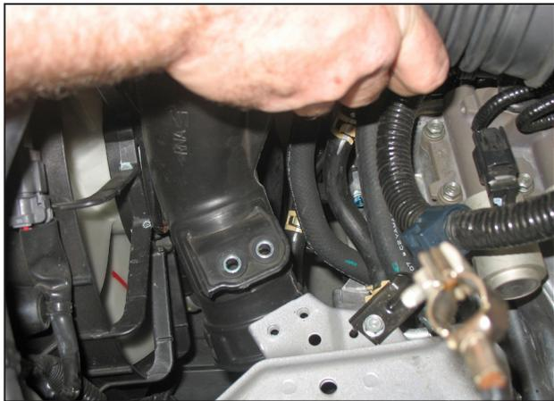
p. Remove the two bolts securing the lower inlet tube to the vehicle.
