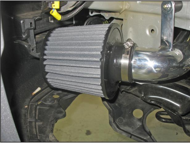
p. Secure the AEM® air filter onto the end of the lower intake pipe with the #9444 hose clamp. Position the intake pipes for best fitment and tighten all hose clamps and rubber mount assemblies.
