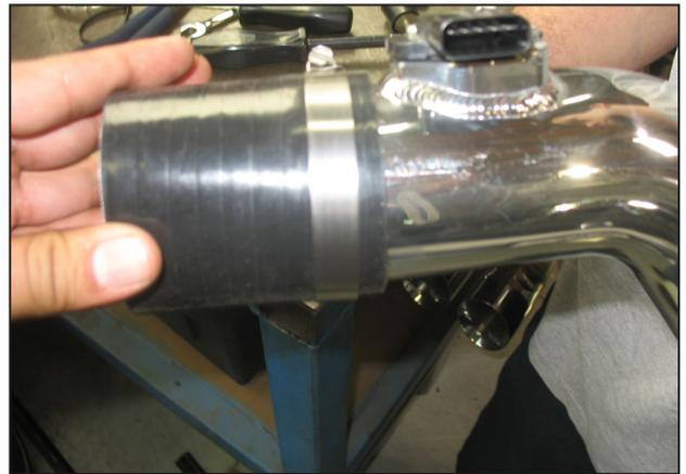
g. Install the 2.50" X 3.00" silicone hose onto the upper intake pipe as shown.
