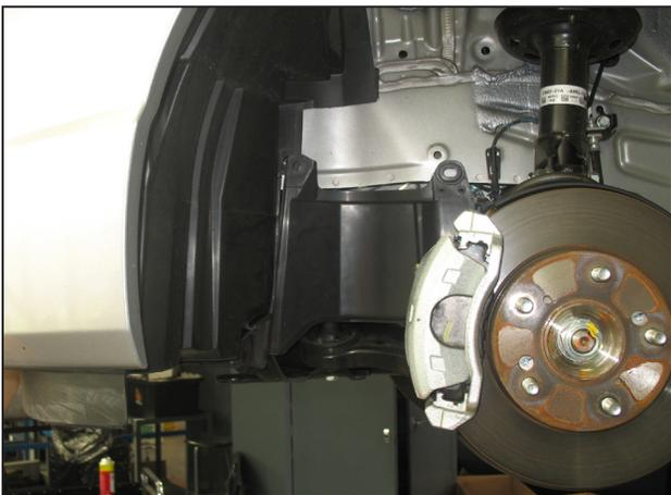
q. Raise the front of the vehicle with a jack. Refer to your owner's manual for proper jack and jack stand placement to properly support vehicle. Support your vehicle using properly rated jack stands before wheel removal or while working under the vehicle. **NEVER WORK UNDER A VEHICLE WITHOUT USING JACK STANDS.** Remove the front driver side wheel.
