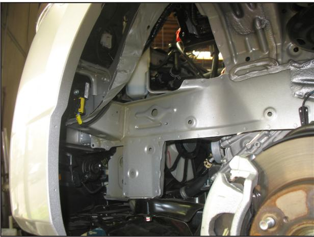
u. Remove the resonator assembly from the vehicle.
