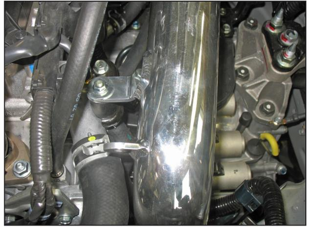
k. Install the washer and serrated nut on the rubber mount to sandwich the bracket.
