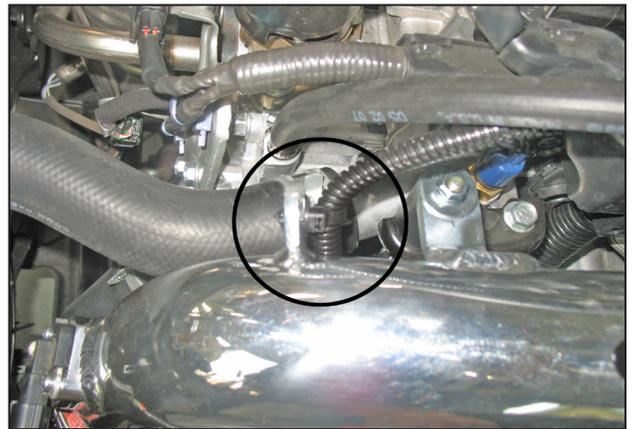
s. Insert the tree-push mount zip tie into the bracket of the upper intake pipe bracket. Secure the MAF sensor harness as shown and trim the excess zip tie. Plug the MAF harness connector into the MAF sensor.
