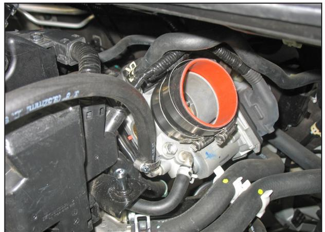
c. Install the 2.50" X 2.00" silicone hose on the throttle body and loosely secure two #9440 hose clamps.
