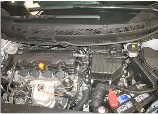
a. Stock air box system installed.
