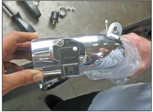
e. Using the stock bolts, secure the MAF sensor to the upper intake pipe.
