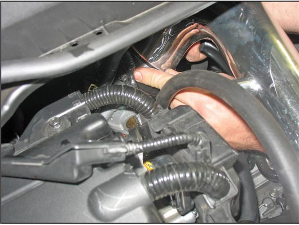
j. Loosely tighten the #9440 hose clamp to secure the intake pipe onto the throttle body.
