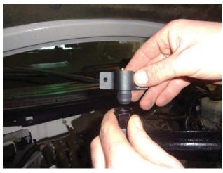
17. Thread the adapter to the top of the tube, but leave the nut loose at this time.
