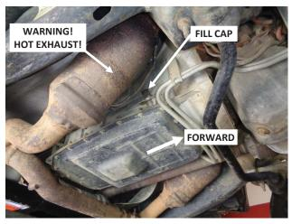
4. Under the vehicle, locate and remove the transmission fill cap. (It is located on the passenger side of the transmission, above and toward the front of the pan.) WARNING: The exhaust system is extremely hot. Wear suitable gloves and long sleeves to avoid burns.
