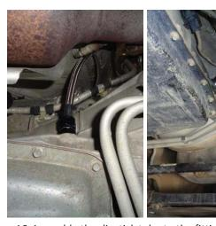
16. Assemble the dipstick tube to the fitting and tighten the nut. **Turn off the vehicle if it is running.**
