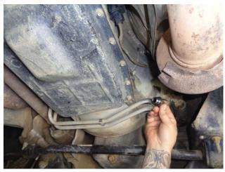
5. Blow or brush off the area around the fill cap, to prevent loose debris from falling into the open port. Then remove the fill cap.
