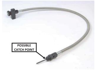
10. Also note if / when the top of the dipstick tip (where it is swaged to the cable) catches on the edge of the fitting (1).
