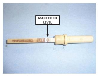
7. Mark the fluid level on the dipstick with a marker or grease pencil and carefully set it aside.
