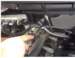
19. Tighten the upper tube nut.
