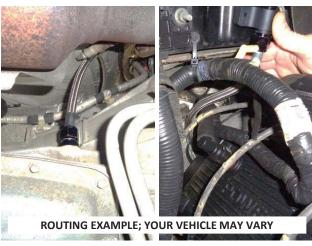
13. Route the tube (2) between the transmission and engine compartment, based on your observations in Steps 9-12.
