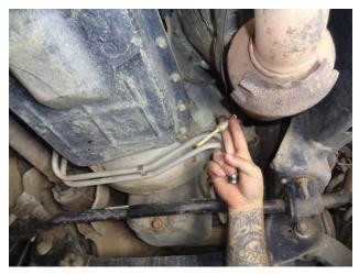
Remove the stock dipstick and wipe it off with a clean rag. Then reinsert it, allowing it to seat fully, and remove it again.
