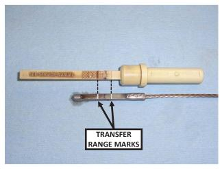
25. Transfer the fluid level range (Max / Min) marks from the stock dipstick to the B&M dipstick. Use a scriber, hacksaw blade or the sharp edge of a needle file to permanently mark the dipstick. Then reinstall the B&M dipstick.
