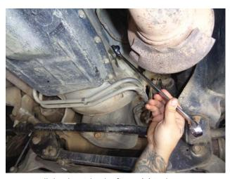
15. Install the dipstick tube fitting (1) in the transmission fill port.
