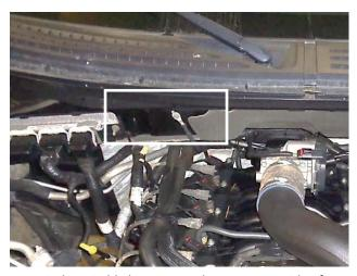
11. Find a suitable location on the passenger-side of the firewall to mount the dipstick adapter (3), while also looking for a suitable route for the dipstick tube.
