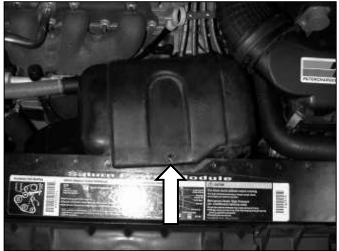
b. Remove plastic clip from resonator and remove resonator.
