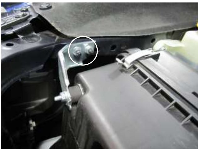
c. Remove the two bolts on the fender that secure the bracket. These will be re-used.
