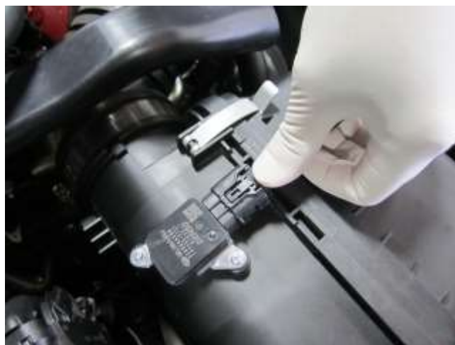
b. Depress the tab on the mass air flow sensor plug and disconnect it from the sensor.
