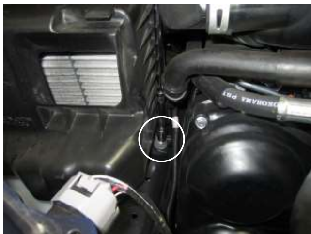
d. Remove the bolt that secures the air box to the engine bay.
