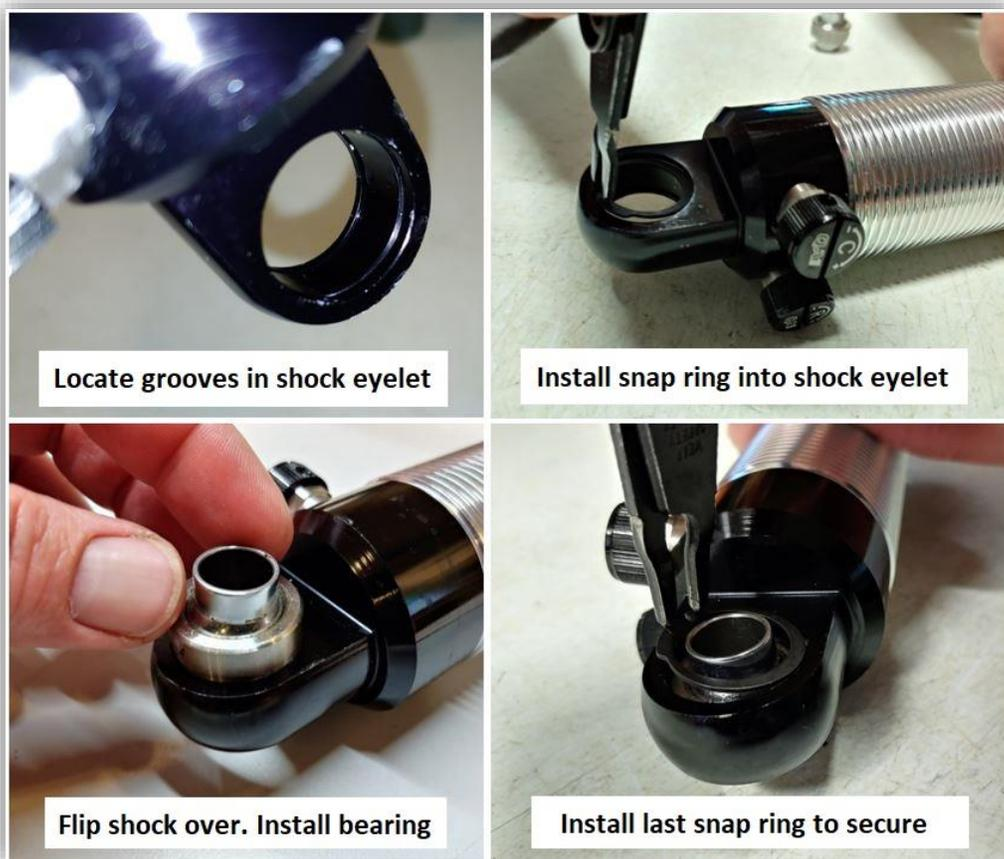
2. Install the coil-over shocks. Torque the lower shock mounting bolt to 70 lb. ft.
